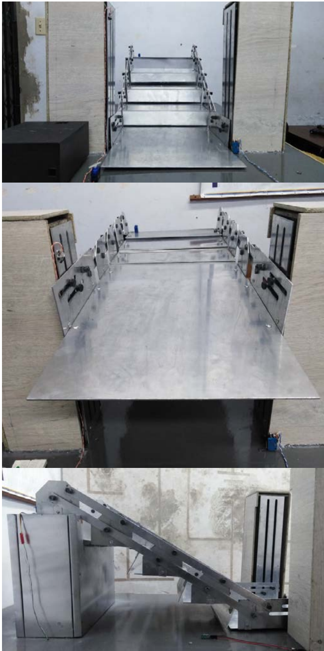
Figure 6. Staircase variation 2 configuring for (Top and Bottom) the first user-type (standard-stairs); and (Middle) the third user-type (elevating platform).
