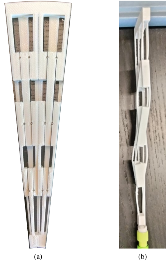
Figure 35: The a) top view and b) actuated side view of the scissor mirror.
