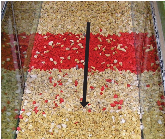
Figure 5a Transported filter material (black arrow indicates flow direction)
