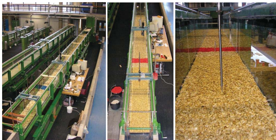
Figure 4: Flume with test set-up in the laboratory at Delft University of Technology
