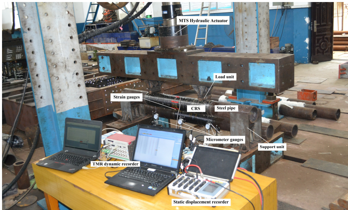
Figure 6.5. Specimen and instruments installation
