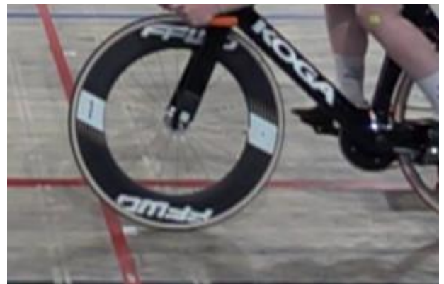
Figure 10 Definition of the distance to the red line. Measured from the centre where the wheel touches the floor and the furthest point of the red line.
