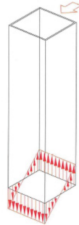
Figure 4-14: Normal stress distribution due to wind load
