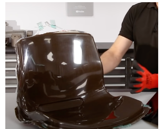
Figure 74 - One of Bcomp's flax reinforcement fabrics (left) (ampliTex™ - Bcomp, n.d.), IB2 Epoxy Infusion Bio Resin (middle) (IB2 Epoxy Infusion Bio Resin - Easy Composites, n.d.), and an example of a flax reinforced composite chair fresh out of the mold (right) (Easy Composites Ltd., 2024).
