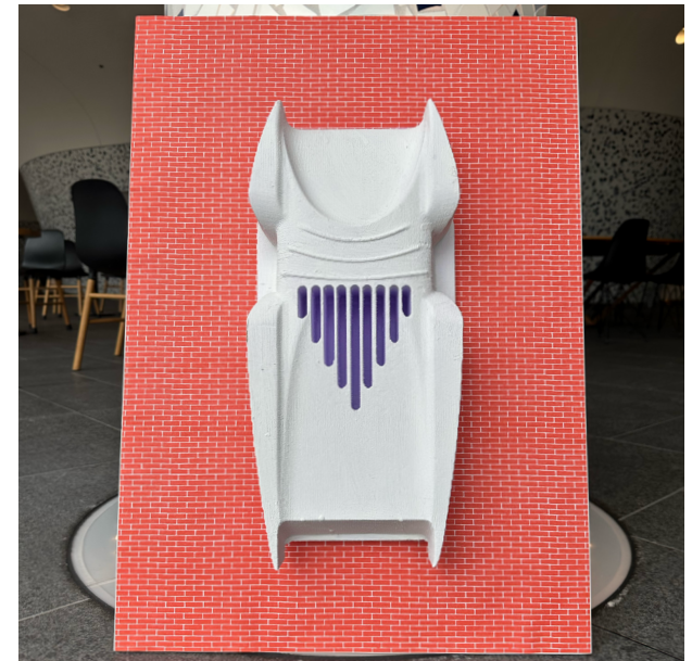
Figure 100 - Foam model with initial front opening design and corresponding DC unit elements. The mill bit was too big to be able to accurately recreate concave ends of the slits.
