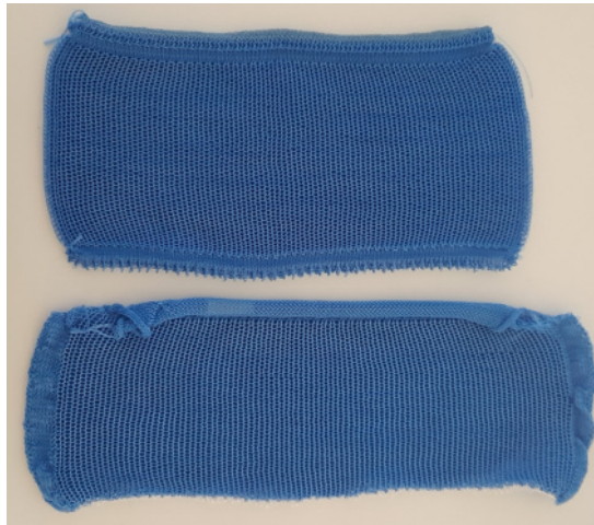
Figure 6.2: Size comparison 100x100 pixel tuck fabrics (top: channels on top and bottom, bottom: channels on sides)
