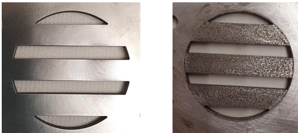
Figure 13 – Comparison of new (left) and used (right) electrode surfaces.
