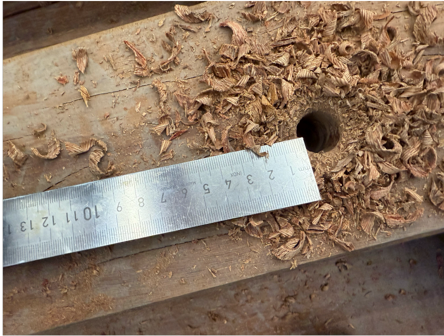
20 mm hole drilled into the lamella
