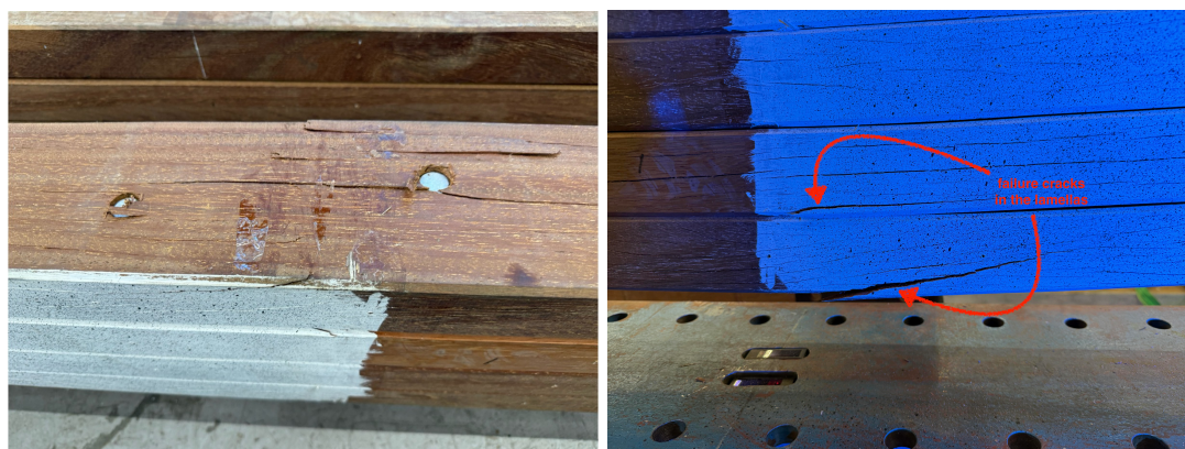
Figure 7.20: Beam B2-2 exhibiting cracks in failure, with rupture at the bottom
