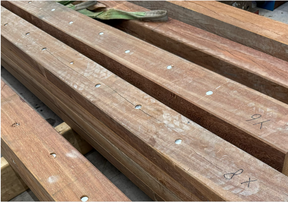
Figure 7.3: dowelled beam B1-1 with running cracks from the dowel holes
