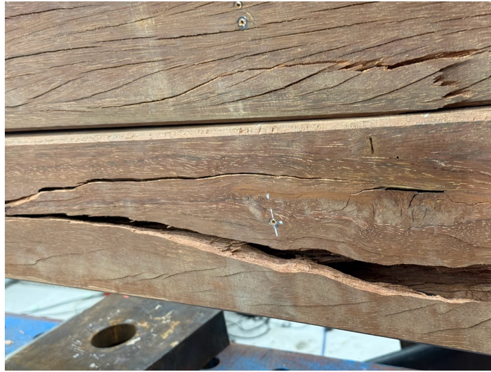
Figure 7.18: Beam A3 after failure
