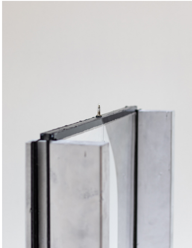
Figure 9.23 | PMMA double sided prototype (author)
