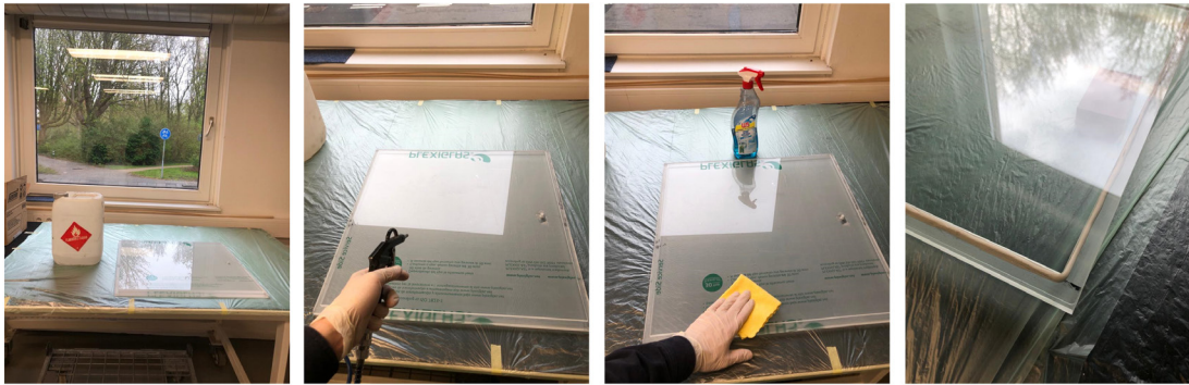
Figure 9.11 | ThinkLab setup: cleaning process with compressed air, alcohol and glass cleaner. Right: PIB seal application (author)
