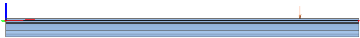
Figure 113 side view numerical model 'De Vecht' with test load at 4 m from the end
