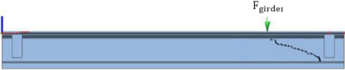
Figure 49 Top: main beam loaded till shear capacity. Bottom: sideview of beam reaching tensile splitting shear
