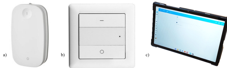
FIG. 5.4 Types of device interfaces used in the experiment: (a) analog light switch, (b) analog roller shade switch, and (c) tablet interface controlling both lights and roller shades.
