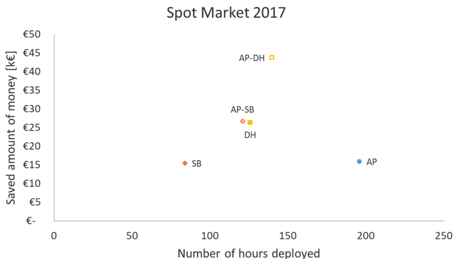
Figure 8.3: Profits that could have been made from the utilisation of an electric heater versus the number of times it could have been deployed for the year 2017.
