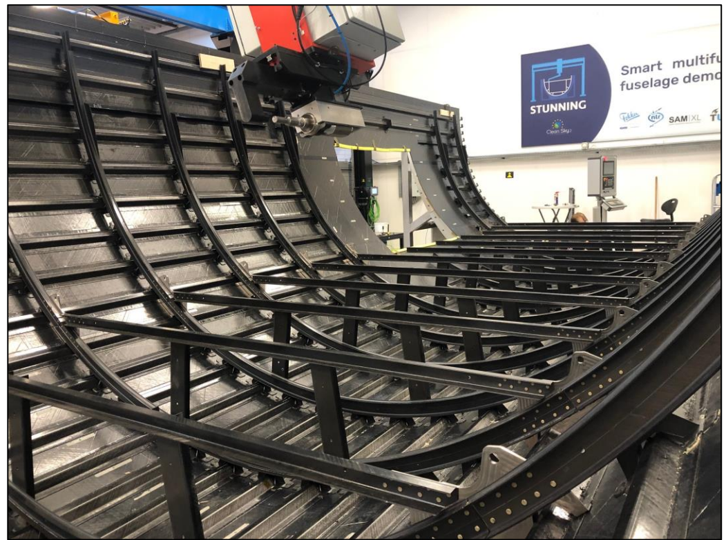
Figure 1. STUNNING demonstrator fuselage, made from welded thermoplastic composites [2]. Project funding source Clean Aviation Joint Undertaking. Photo Credit: SAM | XL. Reprinted with permission from Bram Jongbloed, Project Coordinator. Copyright 2022, Nathan Eskue.
