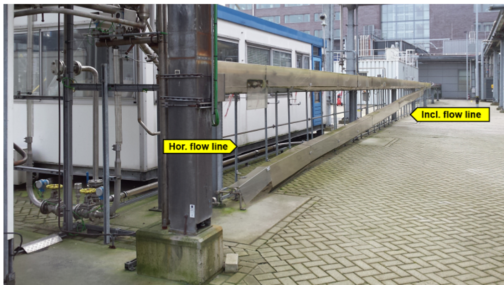
Figure B-5: Second half of the flowline containing the inclined perspex section and the horizontal section towards the T-junction.
