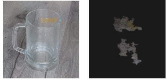
Figure 8: A transparent glass mug; the object to be scanned into a point cloud using Xbox Kinect. The resulting point cloud after the scan (right). It demonstrates that Xbox Kinect is bad at scanning transparent objects.
