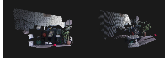
Figure 2: Point cloud scan of a room environment using Xbox Kinect in real-time, shown from two different angles. Demonstrate point cloud's ability to gather environmental information quickly.
