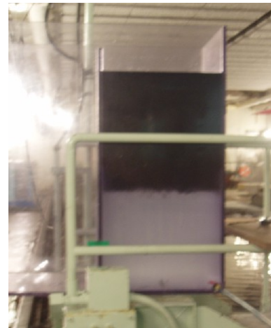
Figure 8. Oil and Water in the Storage Tank
