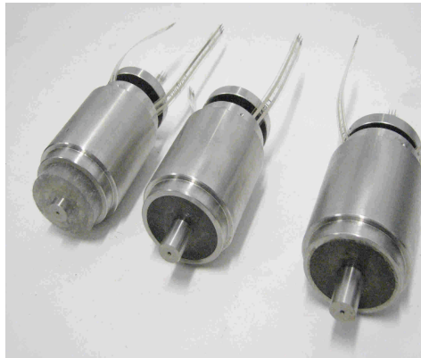
Figure 8. Three samples with three different roughness values are shown after testing. Notice that for sr (left) the ice/cylinder displacement occurred.
