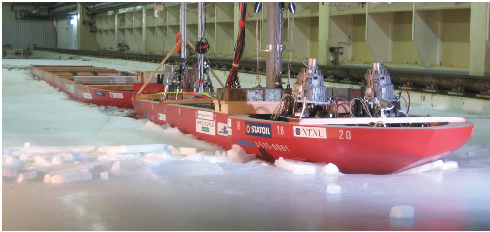
Figure 3 The OIB penetrating a ridge, with the tanker moored in close tow in the background
