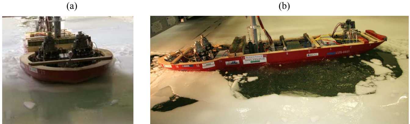
Figure 13 Model testing of the OIB in single mode operation, a) in severe First Year Sea Ice Ridge, b) manoeuvring in ice.
