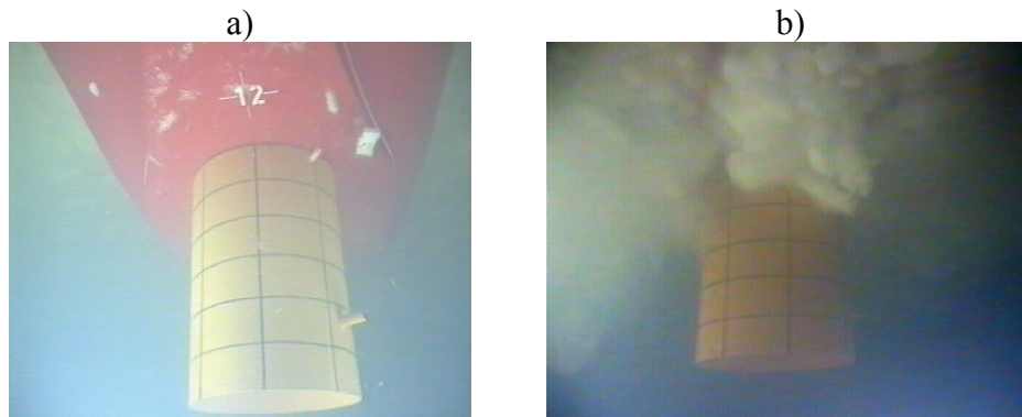
Figure 5 Underwater views of the dummy turret, a) in open water, b) during a ridge interaction (test 4120). The horizontal lines on the bucket are 2 m distant (full scale)
