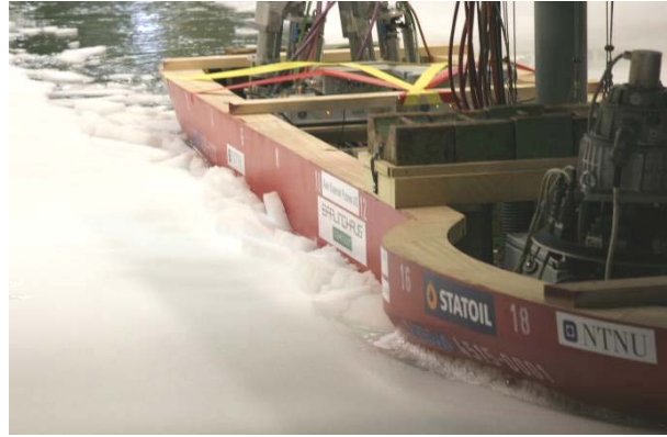
Figure 15 Breaking of level ice by the reamers in level ice
