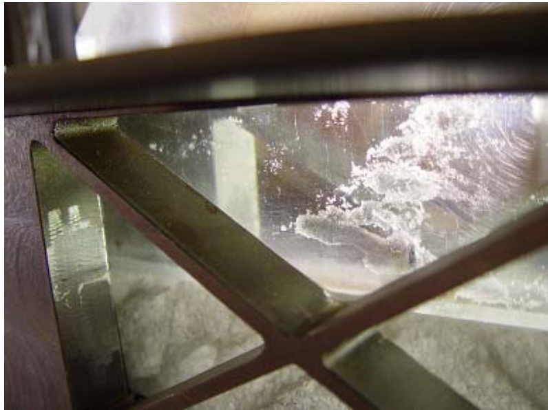
Figure 10. A thin layer of refrozen melt left on the inside of one of the borosilicate glass plates following a crushing test. The thin ice layer is visible just above the X shape in the photo and extends towards the upper right. The changing horizontal location of the ice layer on the glass from top to bottom is a rough ‘strip-chart’ record of the horizontal position of the high-pressure intact ice zone at the platen/ice interface as the test progressed.
