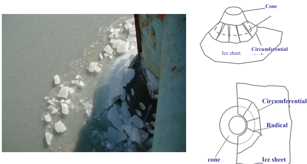
Figure 5. Ice bending failure against a narrow cone.
