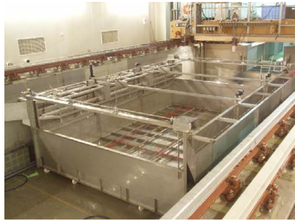
Figure 6. Photograph of Model assembled in Ice Model Basin
