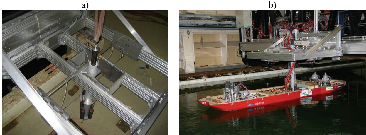
Figure 5 a) View of the mooring frame, b) The dry mooring mounted on the transverse carriage and connected to the OIB
