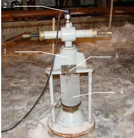
Figure 3. Equipment for the compression tests: hydraulic press (1); pressure gauge (2); displacement gauge (3); ice specimen (4)
