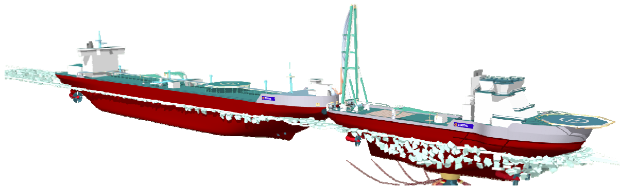
Figure 4 The tested Arctic Tandem Offloading Terminal (ATOT) in close loading mode in ice.
