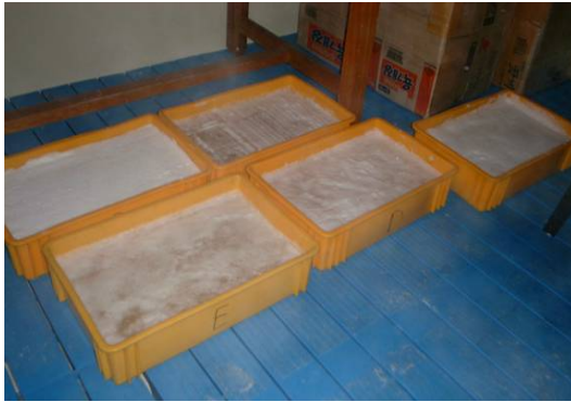
Photo 1. Containers of AG/AD/S mixture solution and the ice specimens cut from frozen model ice solution (Test 1, 2 and 3)
