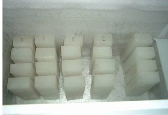
Photo 1. Containers of AG/AD/S mixture solution and the ice specimens cut from frozen model ice solution (Test 1, 2 and 3)
