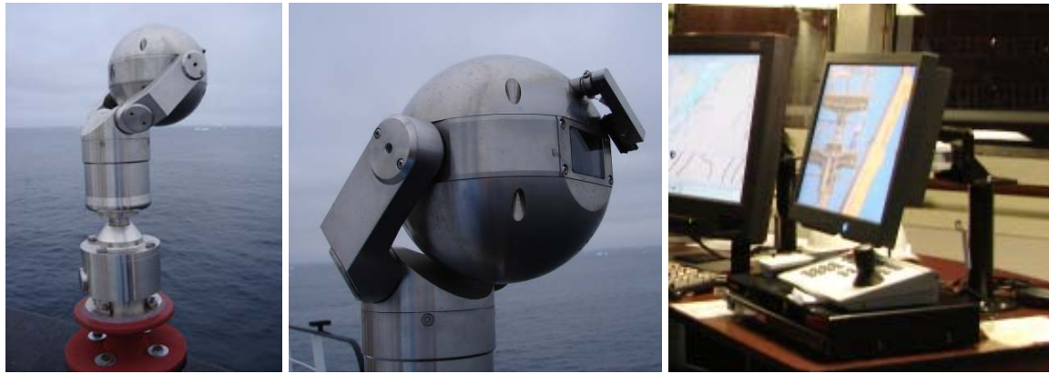
Figure 5. Video camera mounted on the bow of the CCGS Henry Larsen and the video display on the bridge of the vessel.
