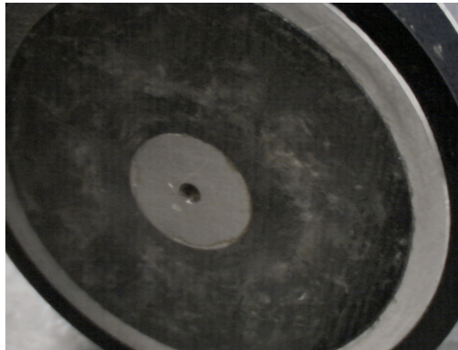
Figure 6. After the ice was cut, the cylinder's and the piston's bottom ends were cleared of ice. Notice the hard plastic ring to protect the connection from the ice formation.
