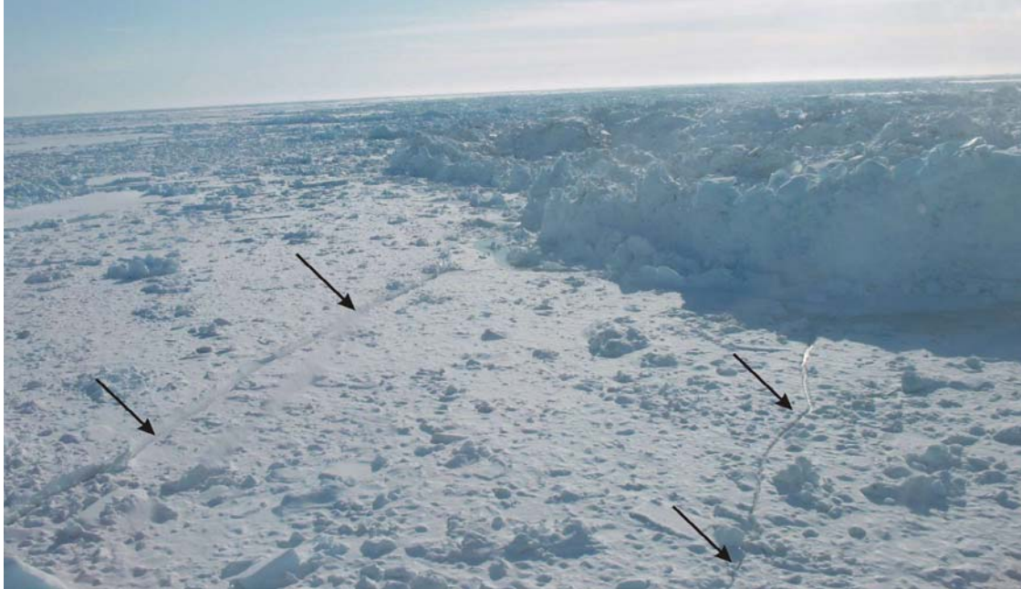
Figure 10. Photograph showing two large radial fractures in the ice sheet as it pushes against a large grounded ice floe.
