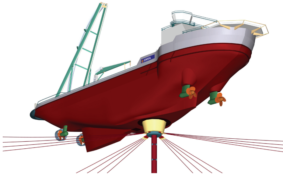
Figure 1 Subsurface view of the Offloading Icebreaker (OIB) moored on its loading buoy. The buoy is connected to a mooring made of 4 clusters and to a protected riser
