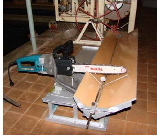
Figure 4. Equipment for ice specimen preparation
