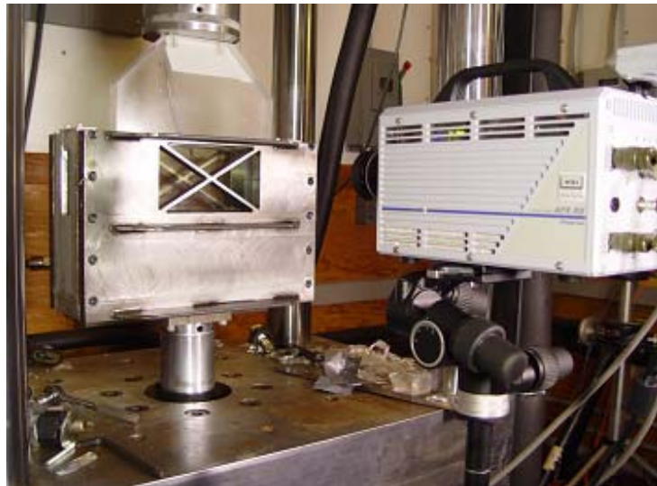
Figure 2. Crushing apparatus and sample mounted in the test frame with the high-speed camera in the foreground.
