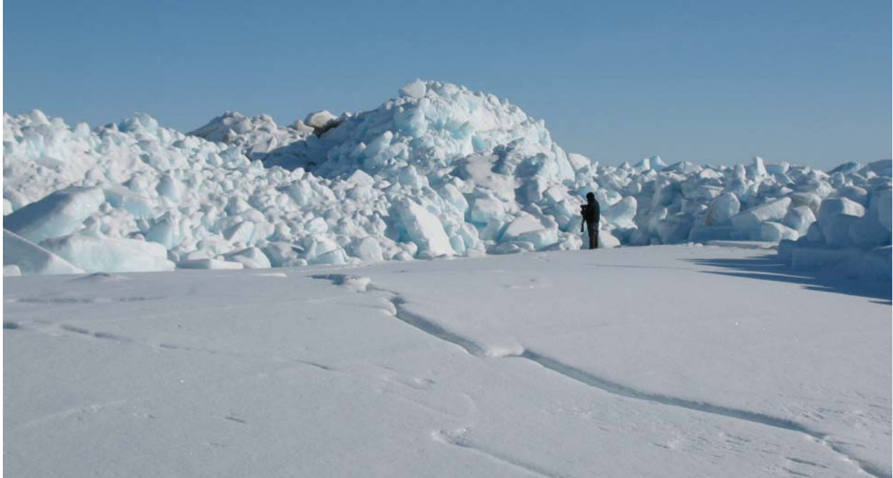
Figure 15. Photograph showing a large pile-up of highly broken ice. Note the crack in the ice in foreground. This ice sheet is “bowed” when it rode up over the ice rubble in a Plate Rafting process. This ice block was more than 0.5 m thick suggesting that this type of plate rafting can take place even with thick ice floes.
