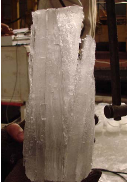
Figure 12. Characteristic picture of ice sample failure
