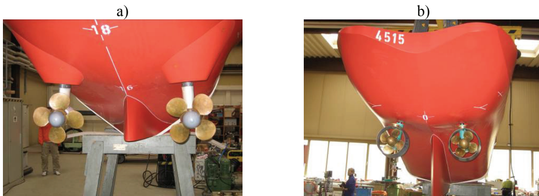
Figure 3 a) View of the bow azimuth propellers, b) View of the stern nozzle azimuth propellers
