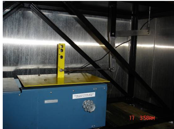
Figure 5. Oscillator and power transfer bar
