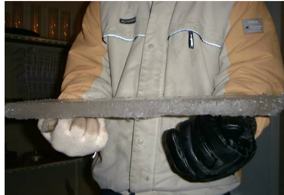
Photo 2. Model ice sheet grown in a small ice tank (Test 4)
