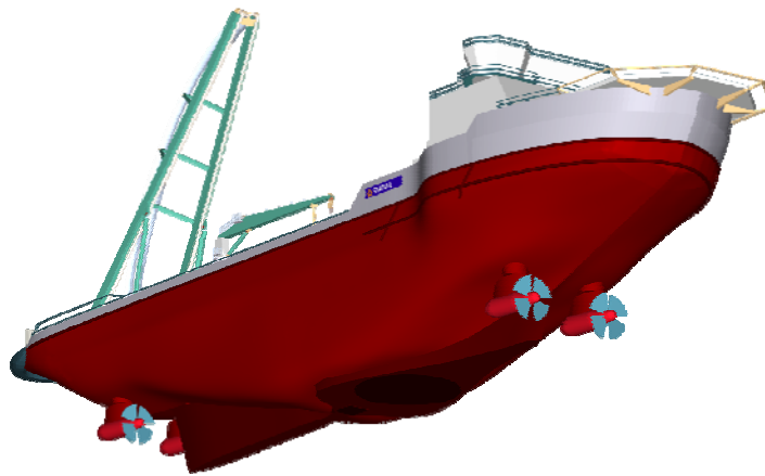
Figure 8 Preliminary OIB hull and propulsion design, 109 m L_{pp} , 21 000 tons displacement.
