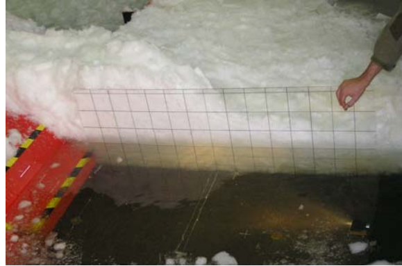
Figure 6. Physical inspection of the ice rubble pile in the centre.
