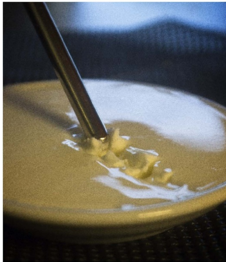
Figure 21. Shear thickening suspension of cornstarch and water. (Left) Photograph illustrating the liquid to solid transition as the surface is scraped (image courtesy of Neil Lin). (Right) Normalised viscosity versus shear rate in experiments and numerical simulations. Reprinted with permission from [313]. Copyright (2015) American Chemical Society. Reprinted from [315], with the permission of AIP Publishing.
