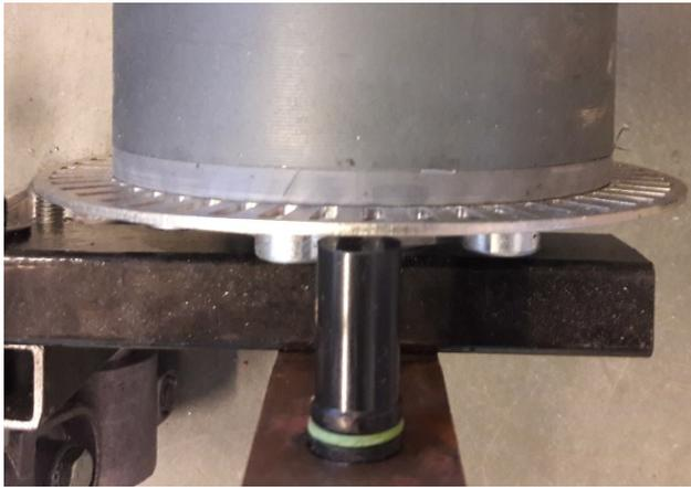
Figure 7.6: Gearwheel sensor mounted at base roller.
