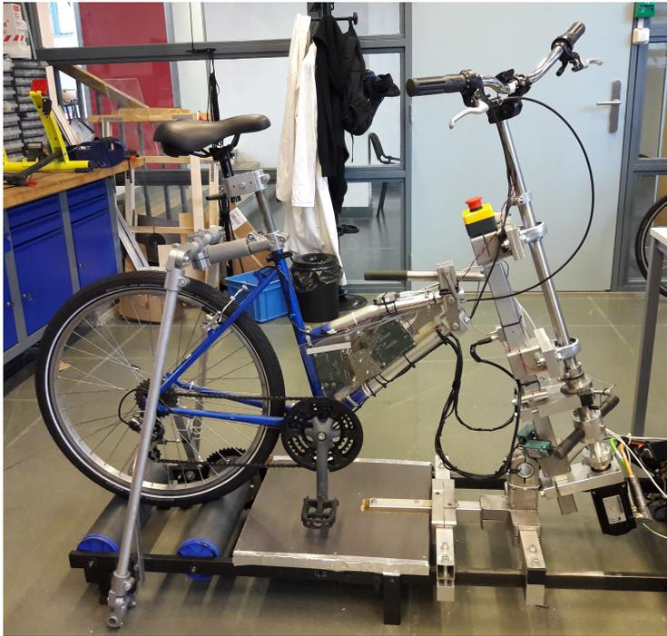
Figure 8.3: TU Delft fixed base bicycle simulator.
