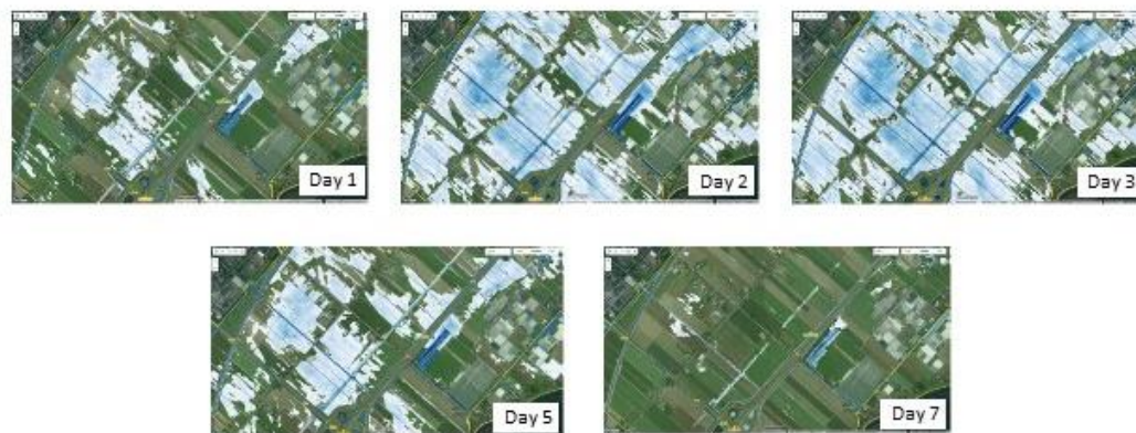
Figure 3: Time evolution of surface water in a spatial section of the “Haarlemmermeer” at day 1, day 2, day 3, day 5 and day 7 of the projected rainfall event (De Bruijn & Slager, 2021).
