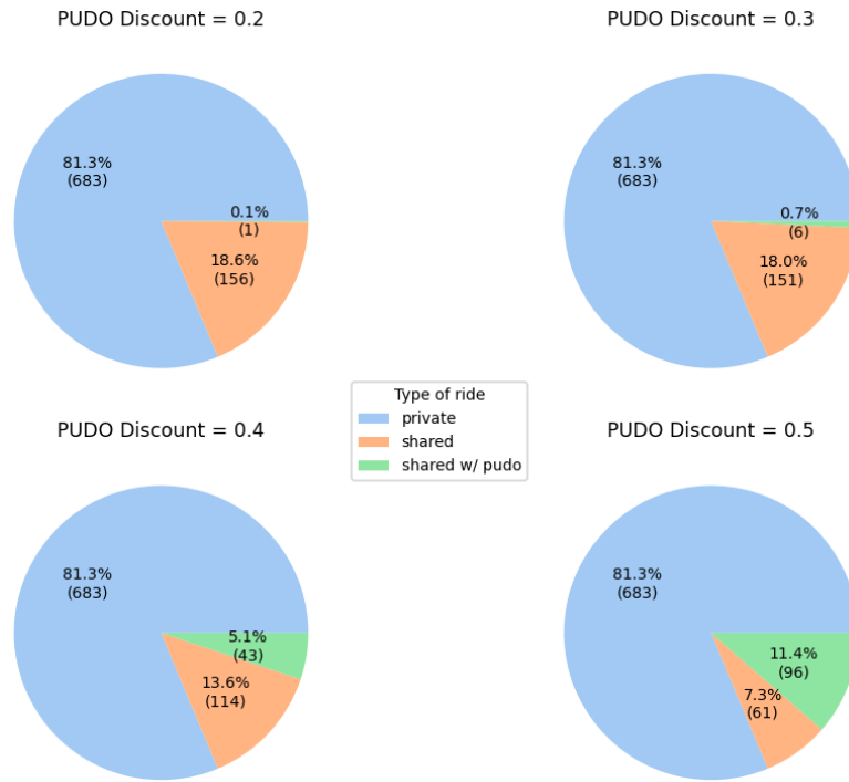
Figure 14: Modal split between private, door-to-door pooled, PUDO pooled rides for a given \tilde{\lambda} when \lambda = 0.2 .
