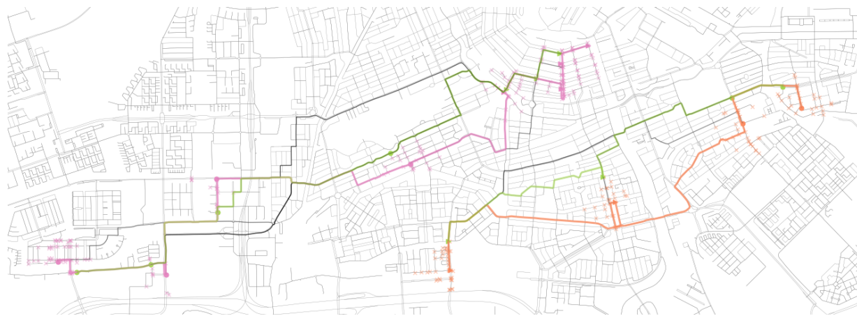
Figure 12: Pooled rides with two and four travellers, visualised by the orange and pink lines respectively where the new route with PUDO points for both is highlighted in green. Dots represent origins while triangles represent destinations.
