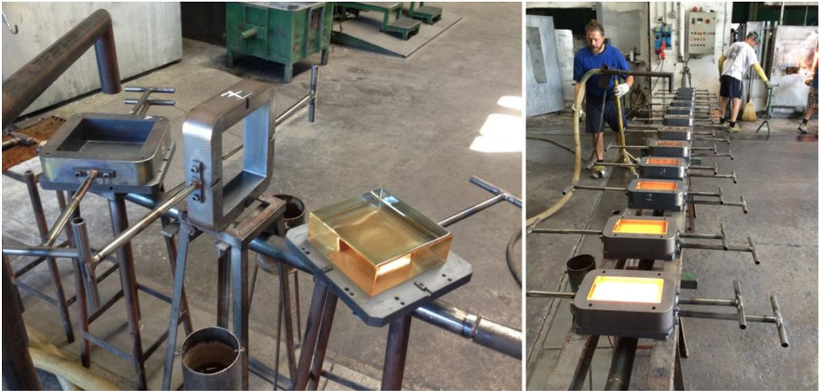
**Fig. 8** *Left:* The high precision, open steel moulds. *Right:* Molten glass bricks during the rapid cooling phase from 1200 to ~ 700 °C degrees
