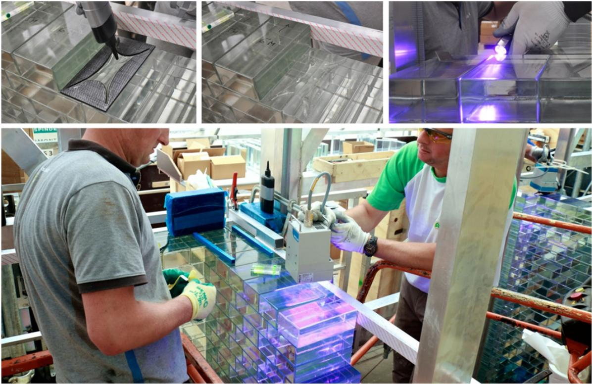
**Fig. 19** Bonding steps from *left to the right*: 1. Application of the adhesive with the aid of the PURE<sup>®</sup> form. 2. Resulting  $\times$  pattern. 3. Local hardening of the adhesive by a UV beam light for
