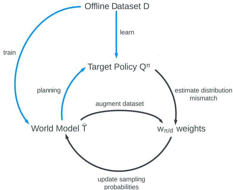
Figure 2: The components of SimuDICE and their interactions. Transitions adapted from Dyna-Q [34] are in blue, while those unique to SimuDICE are depicted in black.
