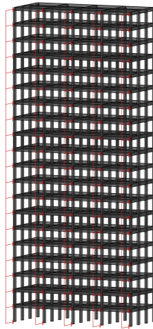
Figure 2.4: Rigid frame system
