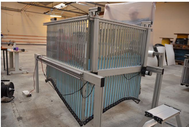
Fig. 15. Form-adaptable boundary wall equipment, to be placed on the flexible table.
