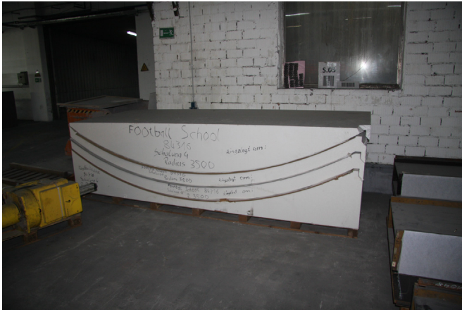
Fig. 4. Single curved polystyrene mould.
