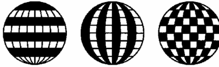
Figure 2.7: From left to right: zonal harmonics, sectorial harmonics, and tesseral harmonics. White areas represent a value above the mean spherical surface and black areas represent a value below the mean spherical surface [32].
