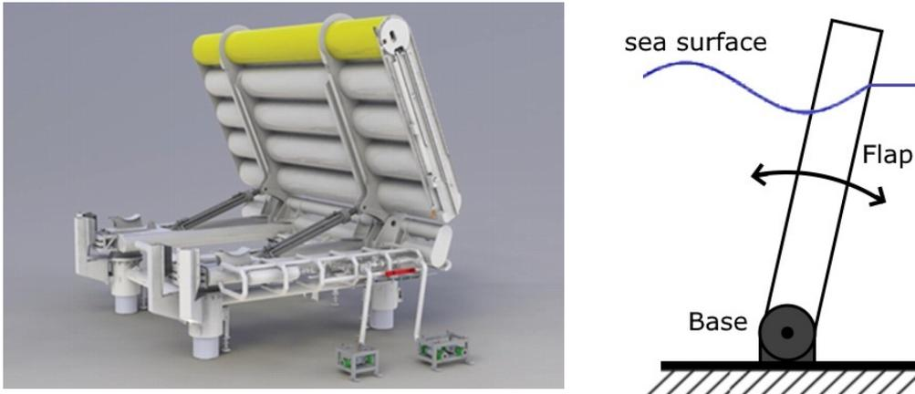
**Figure 2.9:** Model and working principle of the offshore Oyster 1 device [8]
