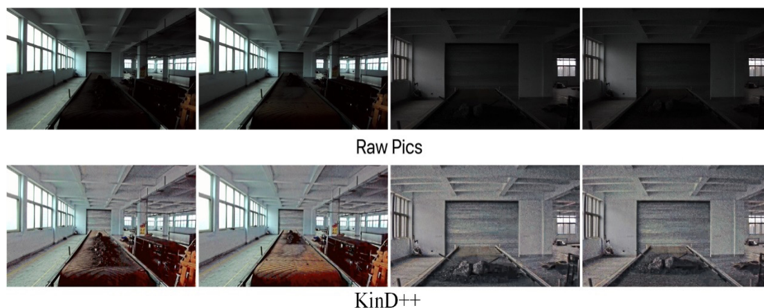
Figure 12. KinD++ algorithm for enhancement of evening without light source image.
