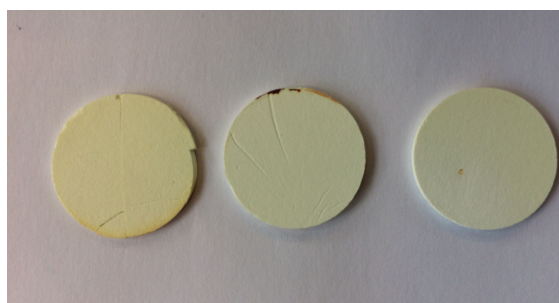
Figure 3.70: Samples taken after 800 °C. Left to right: Zinc Oxide, 6 wt% aluminum oxide doped, 6 wt% aluminum hydroxide hydrate doped
