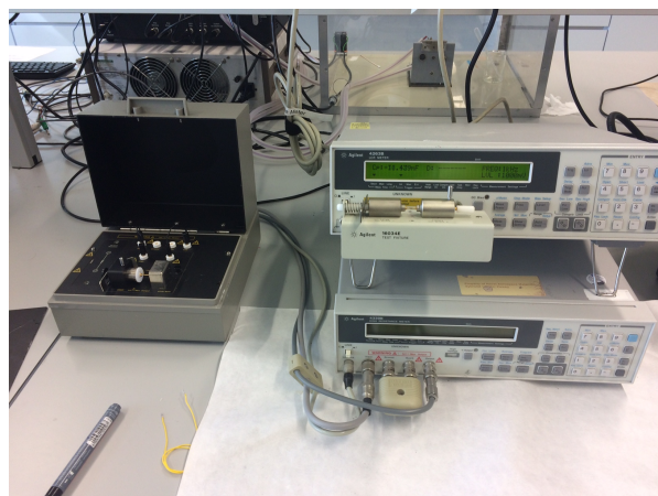
Figure 2.23: Agilent high resistance meter (lower right) and component test fixture (left)
