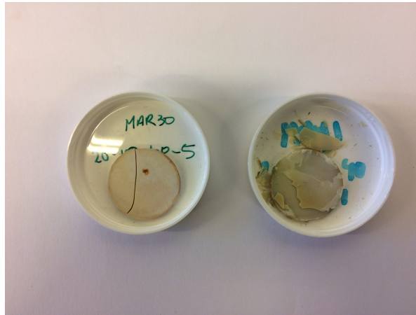
Figure 3.4: Comparison of 150 °C samples to the flaky 165 °C samples
