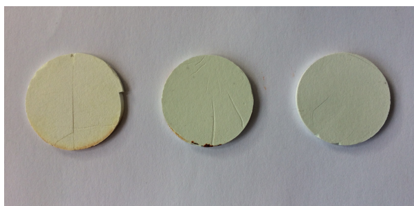
Figure 3.72: Samples taken after 1000 °C. Left to right: Zinc Oxide, 6 wt% aluminum oxide doped, 6 wt% aluminum hydroxide hydrate doped
