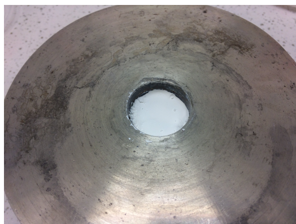
Figure 3.54: Mold with layer of powder in bottom
