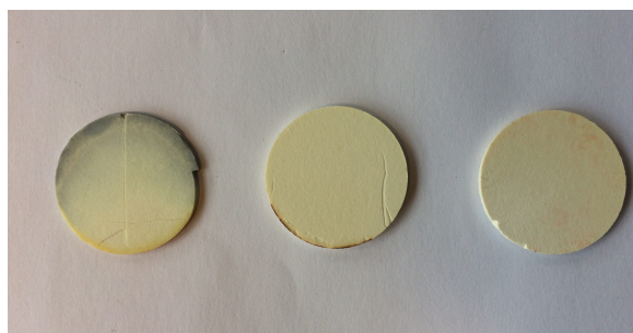
Figure 3.68: Samples taken after 600 °C. Left to right: Zinc Oxide, 6 wt% aluminum oxide doped, 6 wt% aluminum hydroxide hydrate doped
