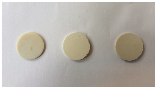
Figure 3.64: Samples taken before the first temperature step. Left to right: Zinc Oxide, 6 wt% aluminum oxide doped, 6 wt% aluminum hydroxide hydrate doped
