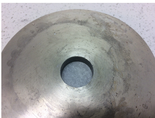
Figure 2.10: Paper circle after fitting of the upper mold
