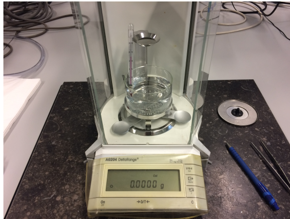
Figure 2.21: Archimedes setup for measuring density
