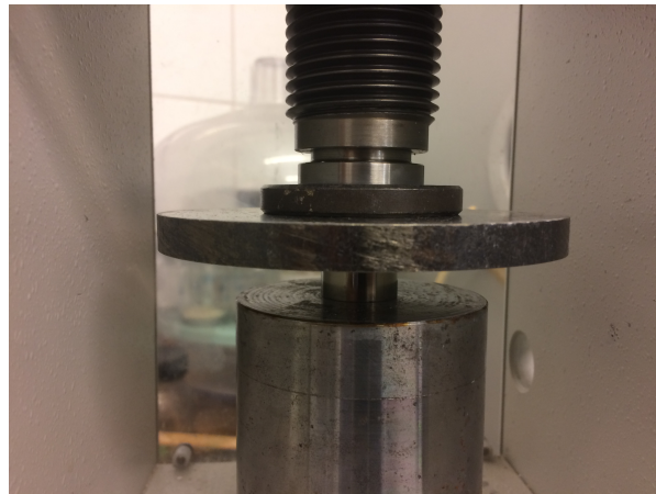
Figure 2.19: Use of washer to remove sample
