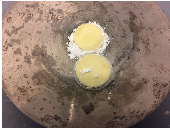
Figure 3.59: Sample after cold sintering process
