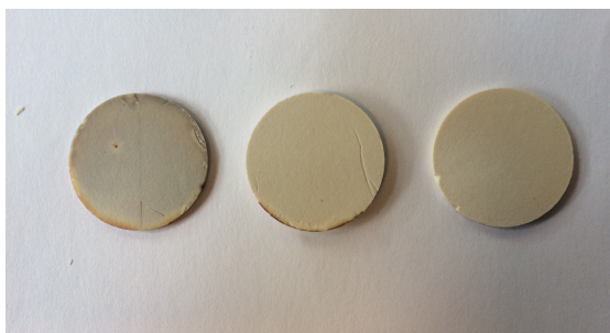
Figure 3.66: Samples taken after 400 °C. Left to right: Zinc Oxide, 6 wt% aluminum oxide doped, 6 wt% aluminum hydroxide hydrate doped
