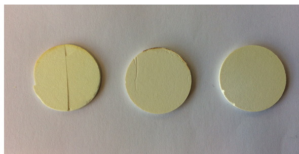
Figure 3.69: Samples taken after 700 °C. Left to right: Zinc Oxide, 6 wt% aluminum oxide doped, 6 wt% aluminum hydroxide hydrate doped
