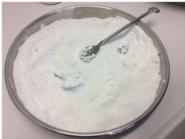
Figure 2.25: Mixing of zinc oxide powder with solution polyethylene glycol
