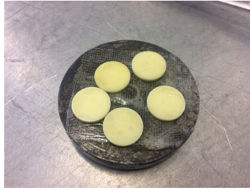
Figure 2.29: Conventional sintered zinc oxide ceramics taped to a steel plate
