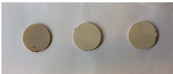
Figure 3.65: Samples taken after 300 °C. Left to right: Zinc Oxide, 6 wt% aluminum oxide doped, 6 wt% aluminum hydroxide hydrate doped
