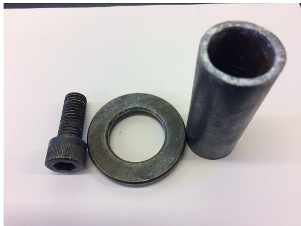
Figure 2.6: Bolt, washer and pipe used to take mold apart after sintering
