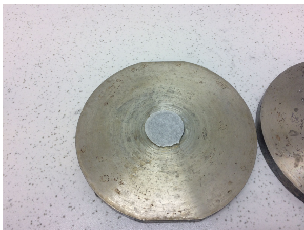
Figure 2.9: Placement of the baking paper circle
