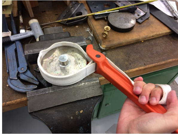
Figure 2.5: Use of the Bahco plastic strap wrench in opening the mold after sintering
