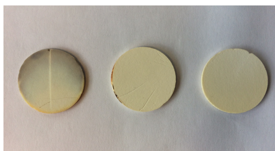
Figure 3.67: Samples taken after 500 °C. Left to right: Zinc Oxide, 6 wt% aluminum oxide doped, 6 wt% aluminum hydroxide hydrate doped
