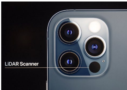
Figure 1.32: LiDAR scanner on an iPhone (Apple, 2022).
