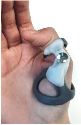
Figure 3.19: Creating a hinge with Chicago screws.
