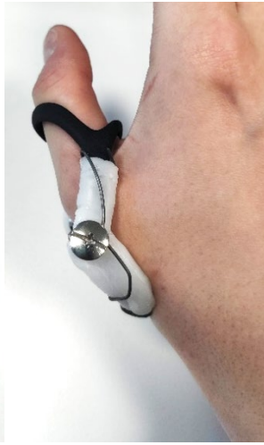
Figure 3.20: Integrating spring steel parts.
