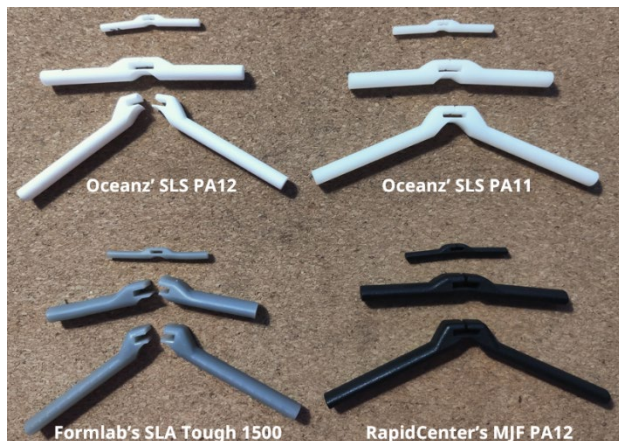
Figure 3.24: A selection of the prototyped hinge samples.
