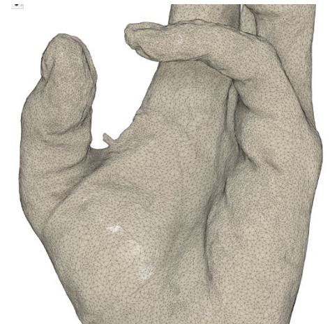
Figure 5.7: Complexities added to the 3D scan geometry around the webspace and thenar muscles.
