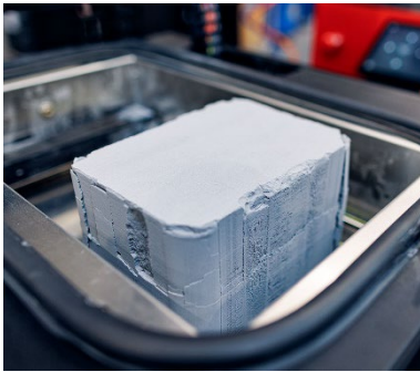
Figure 1.46: The result of SLS (powder bed) printing before cleaning.
