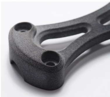
Figure 1.47: The cleaned result of MJF (powder bed & fusion) printing.
