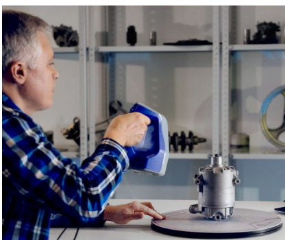
Figure 1.33: The Artec Eva handheld scanner in use (McMillion, 2022)
