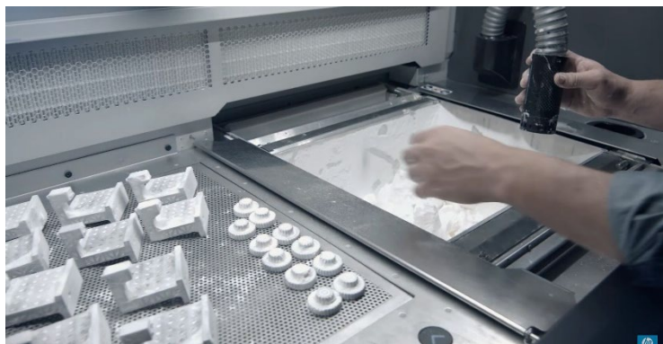
Figure 1.48: Result of MJF (powder bed & fusion) printing being cleaned (HP, 2022).
