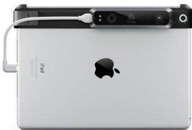
Figure 1.31: Laser triangulation tool in an iPad add-on (Structure.io, 2022)
