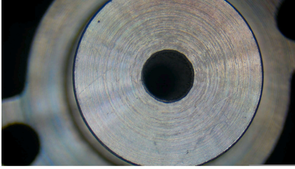
(a) Front view of the resonator inlet after post-machining. The 3 mm diameter cavity inlet is in the centre.
