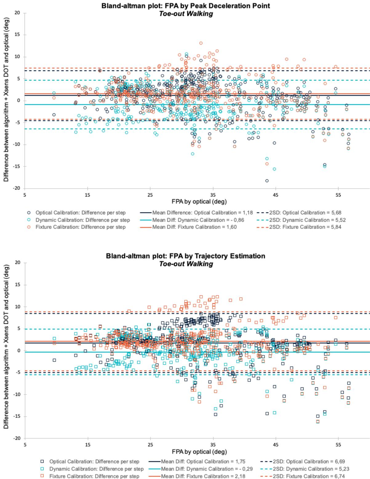
**Figure 10.4:** The mean difference between the algorithms and the optical system for toe-out walking, for three different calibration methods: optical (dark blue), dynamic (light blue) and fixture (orange) calibration method. FPA estimating from the Peak Deceleration Point algorithm is shown in the top graph and the FPA estimating from the Trajectory Estimation algorithm is shown in the bottom graph. Each point represents a step.
