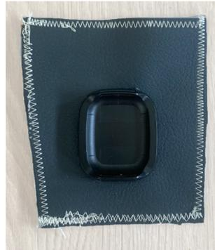
**Figure 5.4:** The sensor-to-shoe fixture: a patch of soft leather with an Movella DOT holder centred
