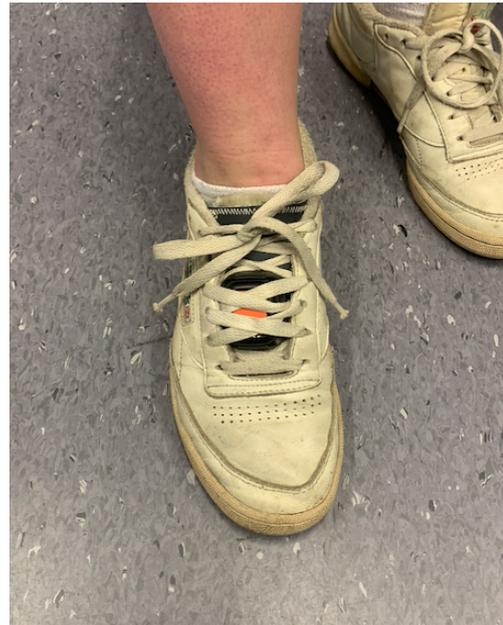
**Figure 11.2:** Participant P4's sensor-to-shoe fixture, displaying a complete fit over the shoe tongue which was not sewn to the shoe body, facilitating accurate alignment with the foot.
