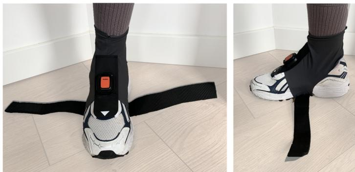
**Figure 5.1:** Sock Concept, for the sensor-to-shoe fixture with the fixation band open, front and side view respectively.
