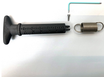
Figure 8.8: Connecting the spring to the handle using a pin (2mm) and hex key.
