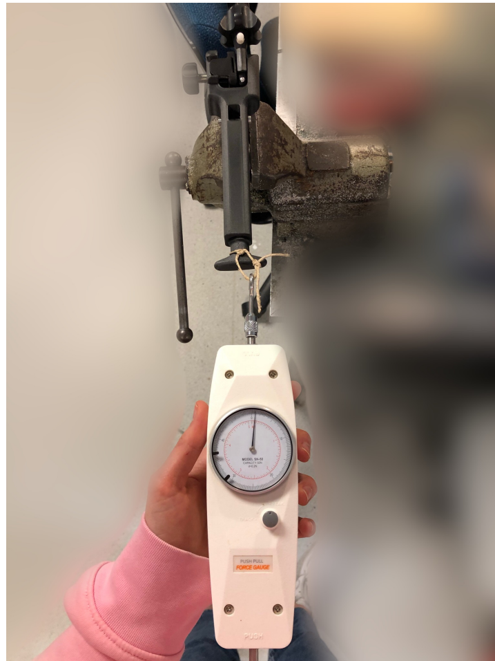
Figure F.2: Assessment of accuracy using force gauge.
