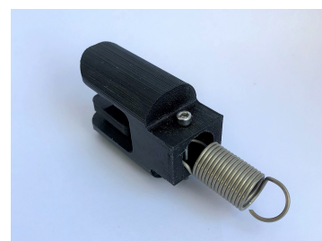
Figure 6.7: Prototype with spring attached using a pin.
