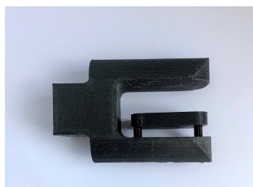
Figure 6.5: First C-clamp prototype with adjustable block.
