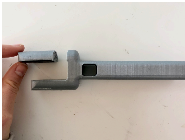
Figure 7.2: Image displaying prototype failure (PLA).
