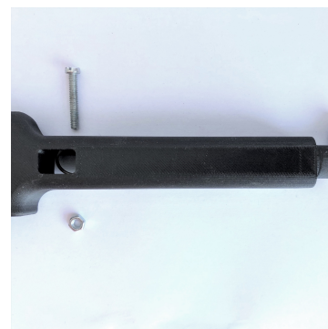
Figure 8.10: Other side of spring connected to the housing using pin and nut (4mm).
