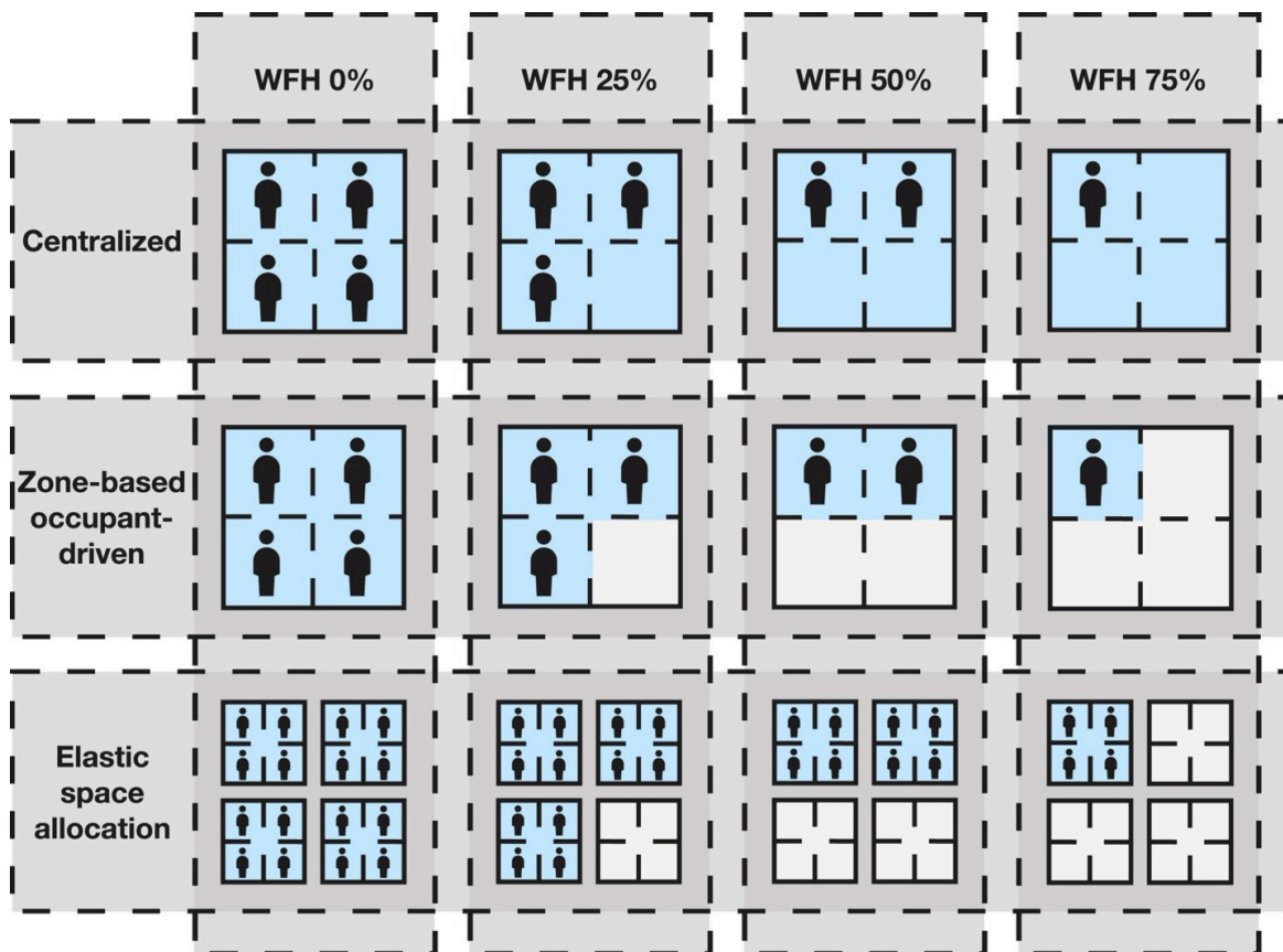
Figure 1: Blue squares represent sections of the building operating their cooling systems. In buildings with centralised cooling, cooling requires the same amount of energy regardless of occupancy. In the other two conditions, cooling systems only switch on when sensors detect occupants in that area of the building (zone-based occupant-driven) or users book the space beforehand (elastic space allocation).
