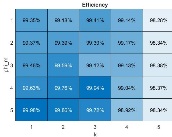
Figure 5-22: A quantitative heat map of the average efficiency of the wing stroke, associated with each of the 25 combinations of attitude control parameters. This figure corresponds to the flow case that simulates the vertical oscillation during hover.
