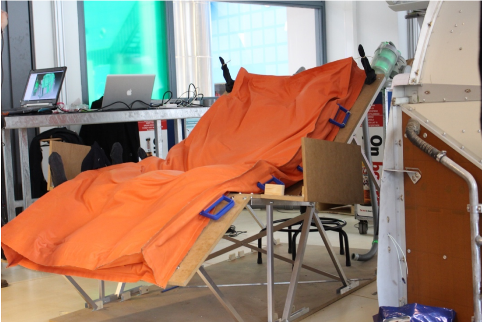
Figure 4.7 | Reference pins on test seat, covered by socks for safety.
