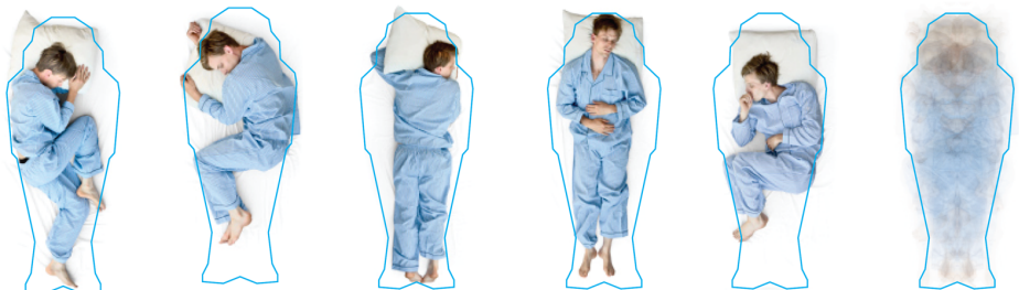
Figure 7.2 | Example of how postures could dictate a minimal space envelope which provides room for postural change and movement. In such a design, anthropometric variation within the target population needs to be considered.
