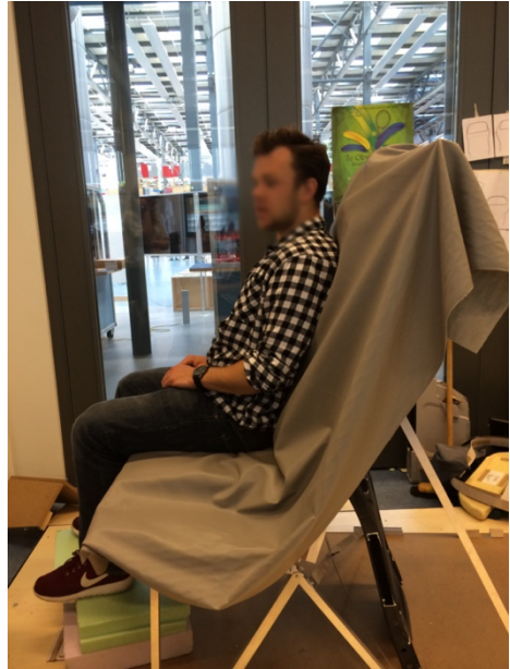
Figure 4.10 | Trial and error test for finding a comfortable cushioning firmness distribution.
