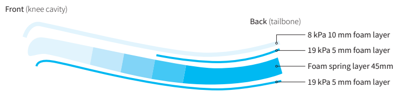
Figure 6.5 | Side-view of the prototype seat pan showing the layer composition of different foams.
