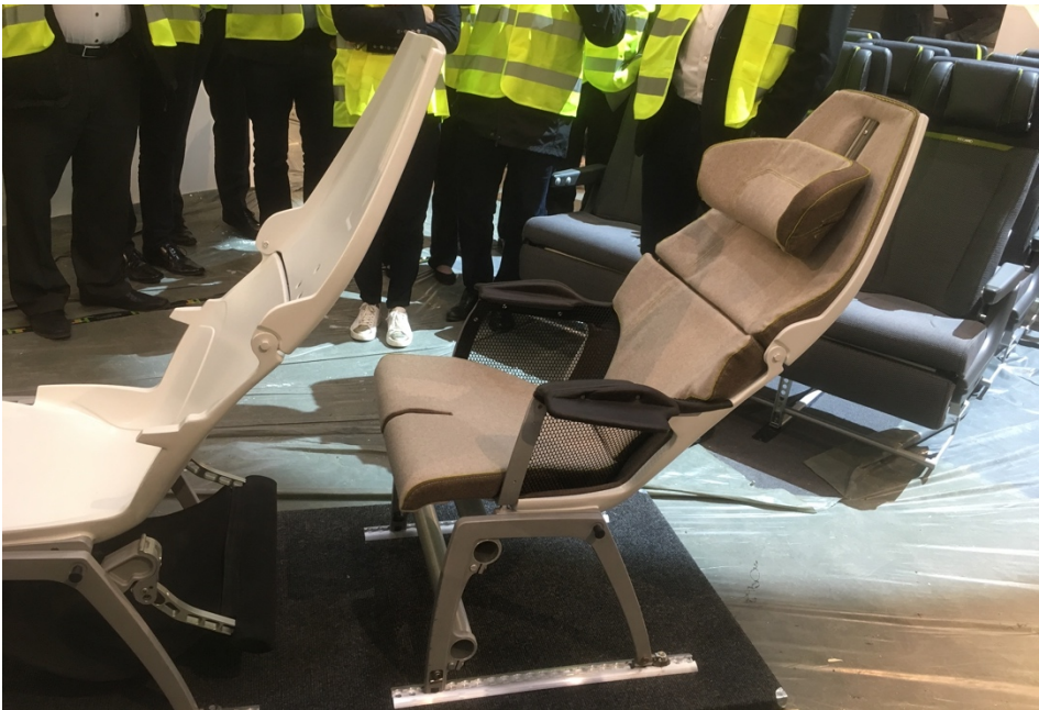
Figure 11.1 | RECARO Aircraft Seating human contour-based prototype seat (left) as presented at the Aircraft Interior Expo 2019 in Hamburg, Germany. The double curved backrest provides additional (knee) space for the occupant behind the seat. Photo by Peter Vink.
