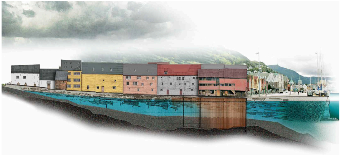
Figure 6: Section of Bryggen with Deposits T. Sponga. Section Showing Buildings, Archaeological Deposits, and Groundwater . Riksantikvaren
