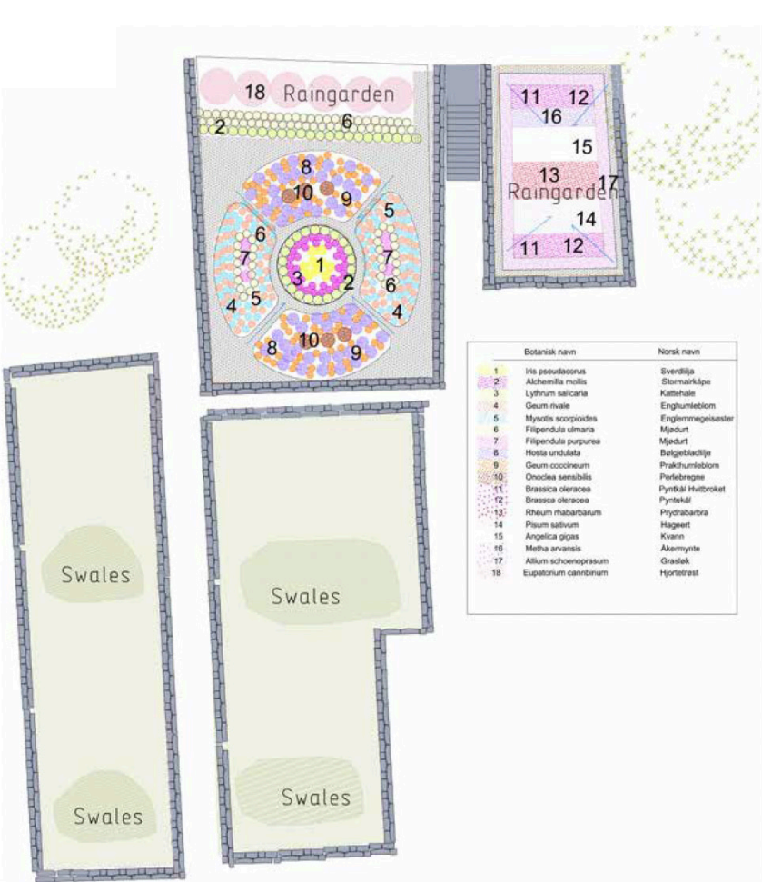
Figures 9-10: SUDS Strategy Drawings of Current Interventions Multiconsult AS. (2017). Cross Section and Schematic of Rainwater Garden. Riksantikvaren.
