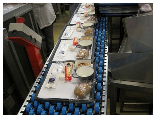
Figure 2-5 - ICA-M food assembly line
