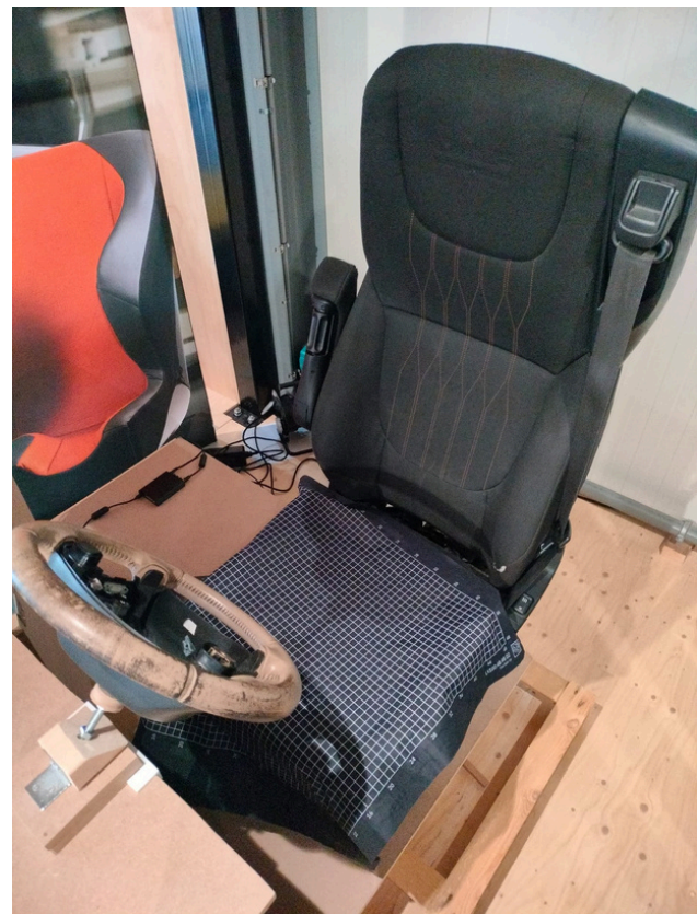
Figure 35: The truck seat covered with a pressure mat during testing
