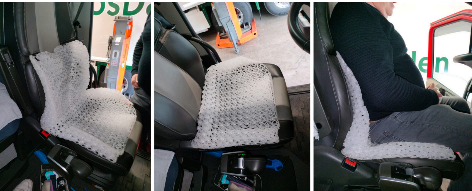
Figure 11: The concept being tested in a Volvo Globetrotter XXL, with the truck driver it was tailored to
