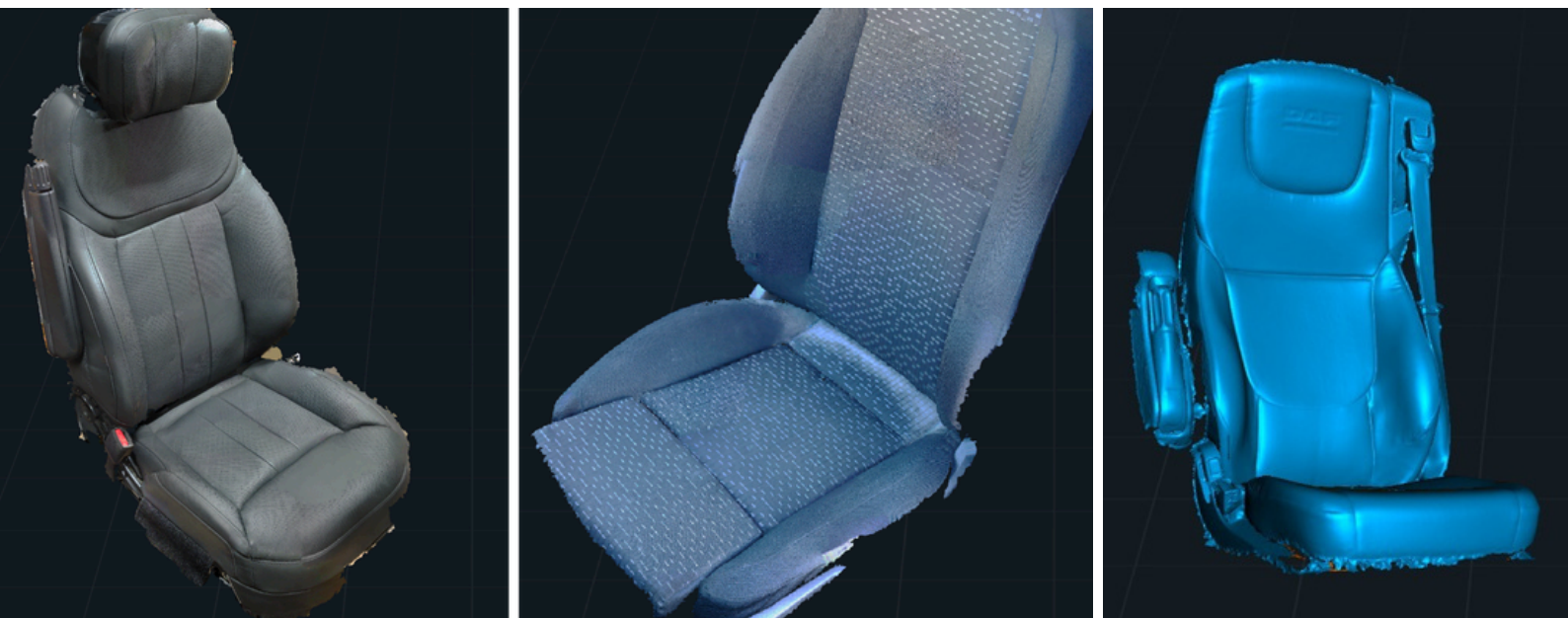
Figure 15: Scans of different car seats, made with the Creality Ferret SE
