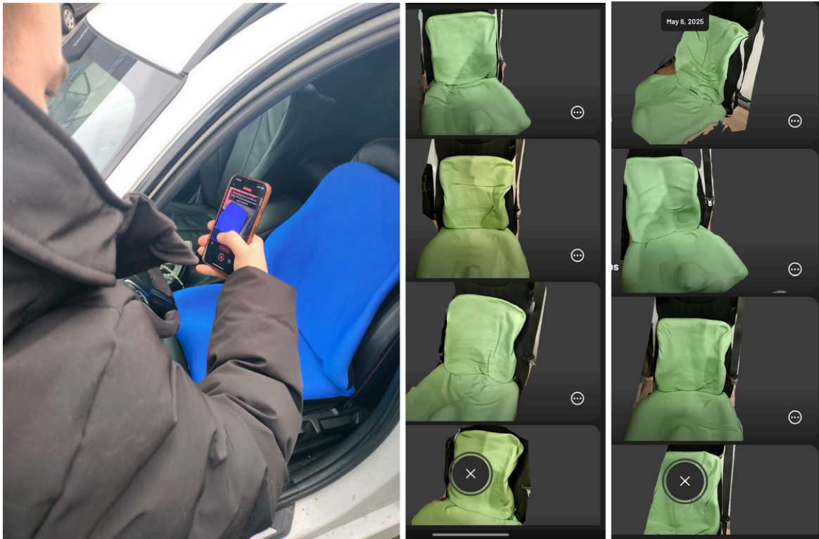
Figure 16: Scanning with the Scaniverse app and its results
