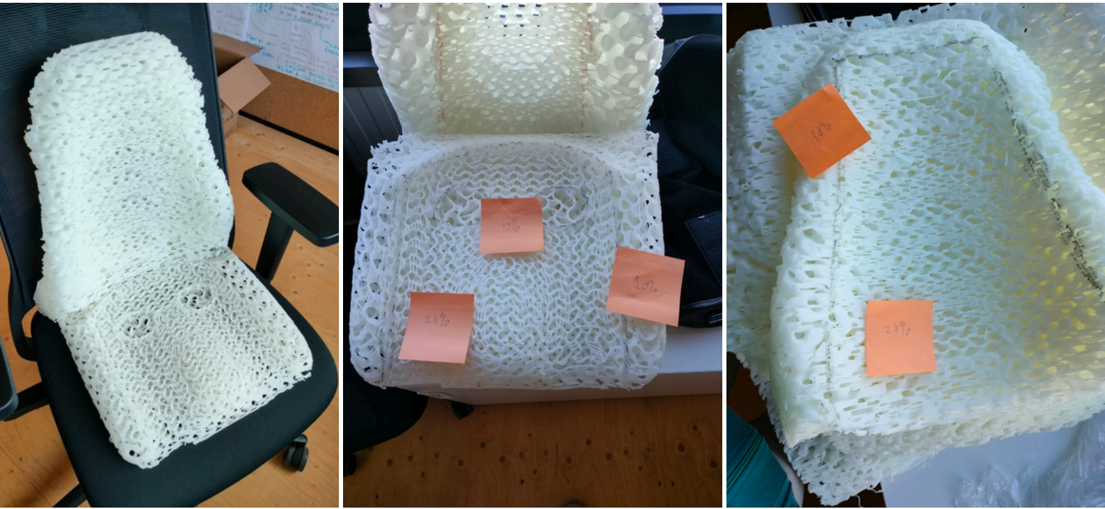
Figure 5: Small Two Part concept shown with infill percentages and split up
