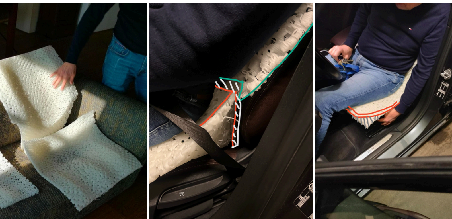
Figure 8: The XL Two Part concept being tested with an occupational driver
