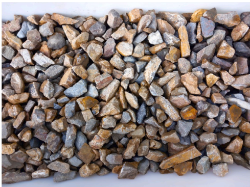
c Clean ballast particles in the reservoir: AREMA No. 4
