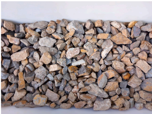
d Clean ballast particles in the reservoir: AREMA No. 4A
