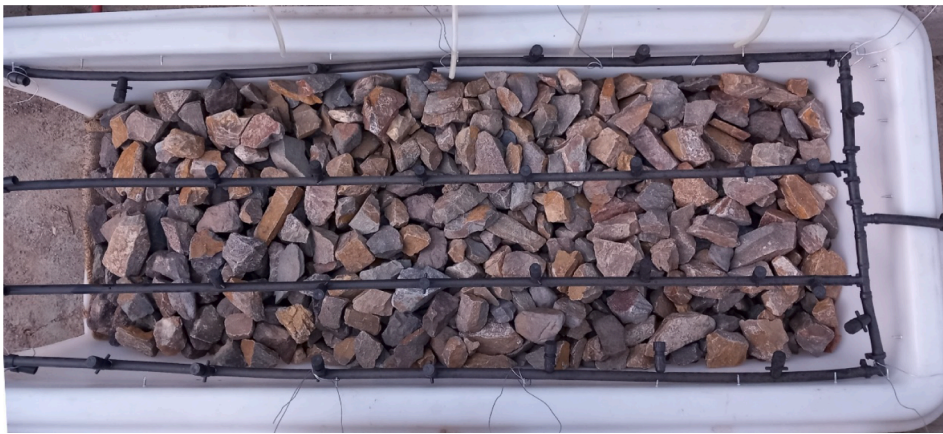
a Reservoir and rainfall generation system
