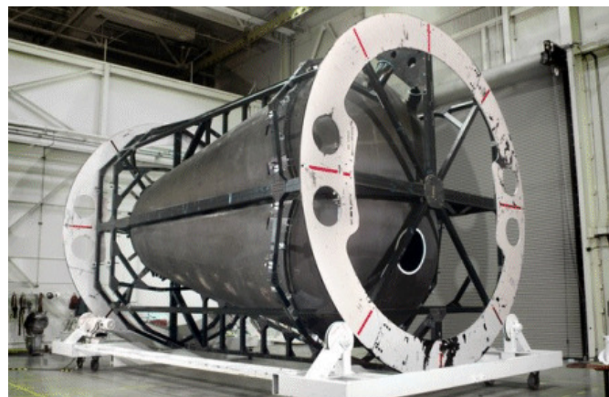
Figure 2.7: X-33 Composite Sandwich Tank [52].
