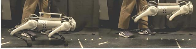
Fig. 1. Delft E-Go, the compliant quadruped with parallel elasticity, stores energy in springs (left) and releases it for an explosive jump (right).
