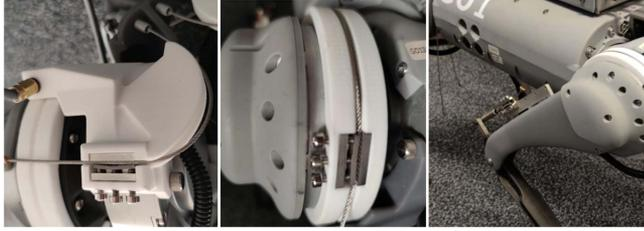
**Fig. 4.** Installation of the spring engaging mechanism: left is for the hip joint, middle the thigh joint, and right the calf joint.
