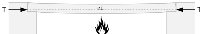
Figure 33 | Simply supported, thermally restrained concrete member with the thrust forces
