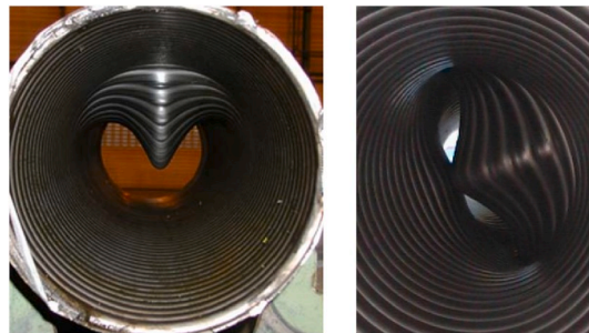
Fig. 3. “Heart” mode (left) [16] and “Eight” mode (right) [17].
