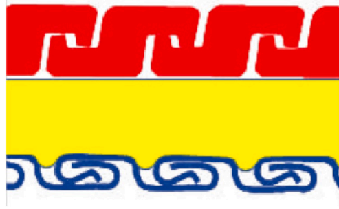
Fig. 2. Extrusion of the liner into the adjacent interlocked carcass [12].
