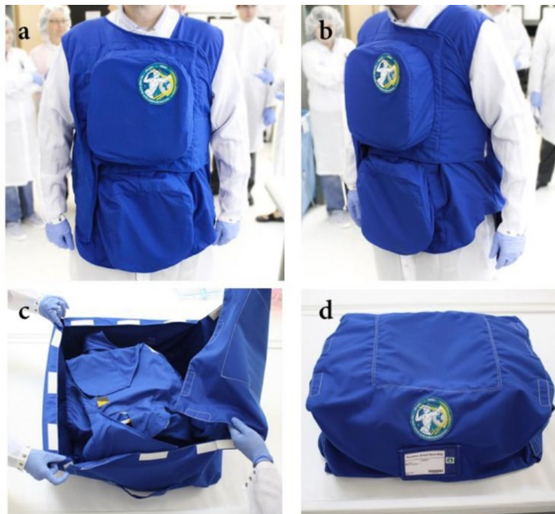
Figure 6: The PERSEO suit for its first ISS test, aimed to assess the suit's operation time for filling and emptying, and the overall astronaut comfort. Source: [24].
