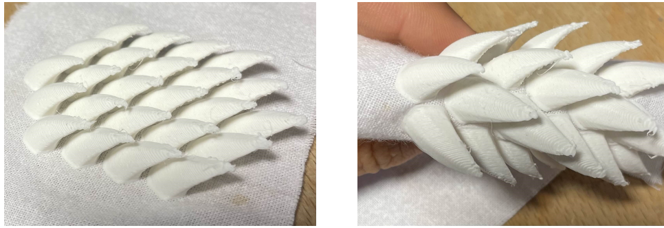
Figure 33: 3D-printed PLA scales on a fabric layer. The left image displays a fabric with PLA scales printed on its surface, while the right image shows the same fabric with scales bent to demonstrate flexibility of a hard material through considerate design. Produced in the Spaceship EAC laboratory with the help of fellow intern Louis Quinot.
