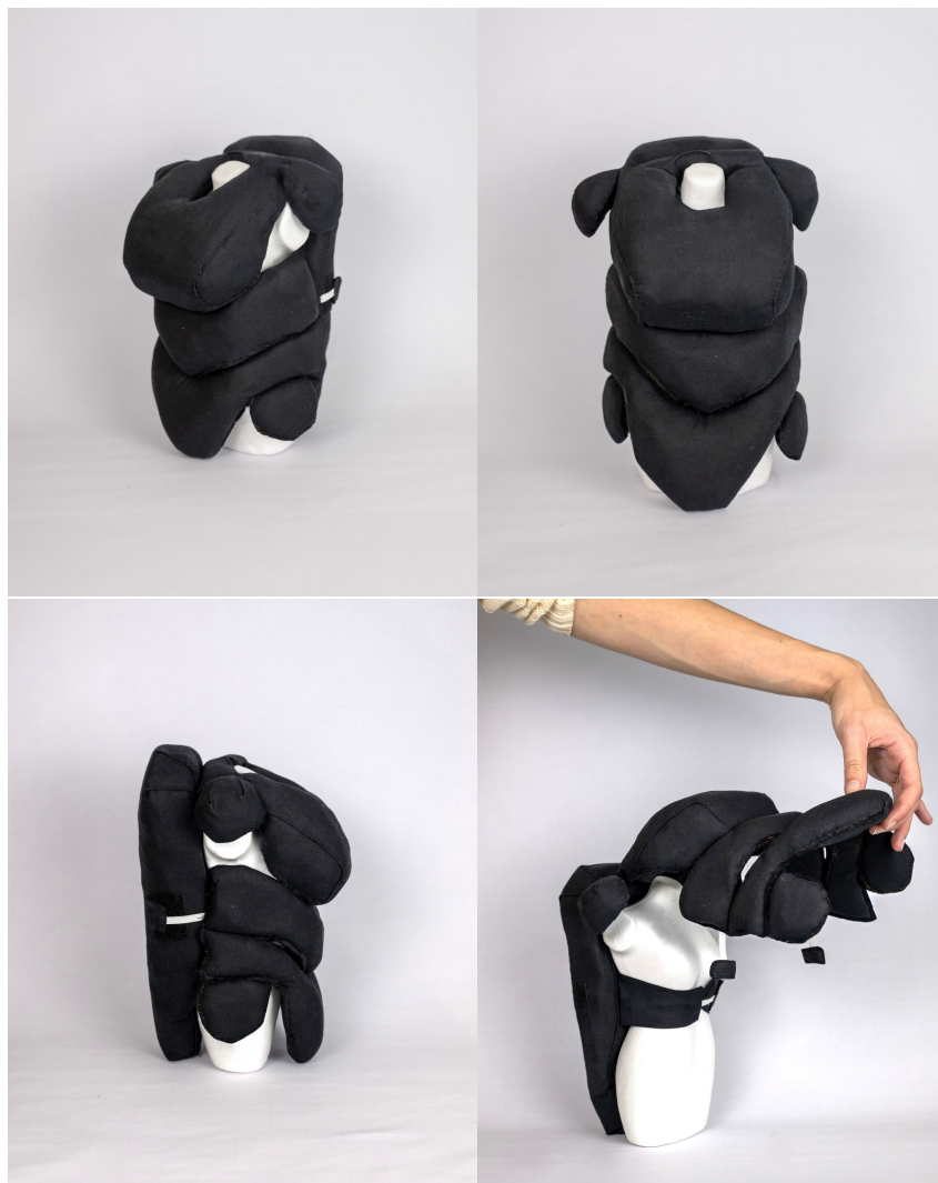
Figure 34: 1/4-scale FLARE suit prototype on displayed on a mannequin from multiple angles. Upper left: angled view showing the suit's overall structure and proportions. Upper right: front view. Lower left: side view. Lower right: shot of the partial donning process, showing the back section secured with a belt at the midsection, which is to be followed by the front flap closure.
