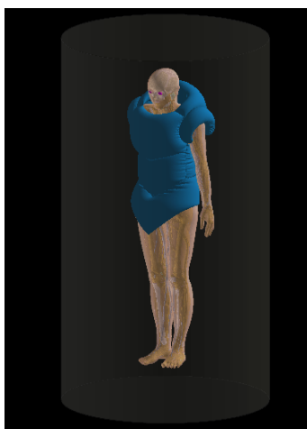
Figure 46: 3D simulation setup, including the I-HAB module (dark grey), FLARE prototype vest (blue), and human phantom.
