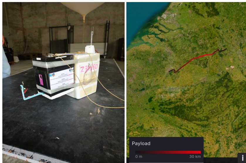
Figure 50: On the left, the SensorConfetti payload is shown before flight, after attachment to the ozonesonde payload of the RMI (white box). On the right, the flight path with altitude label of the payload is shown. The stratospheric balloon was launched in Uccle and landed near the city of Venlo.
