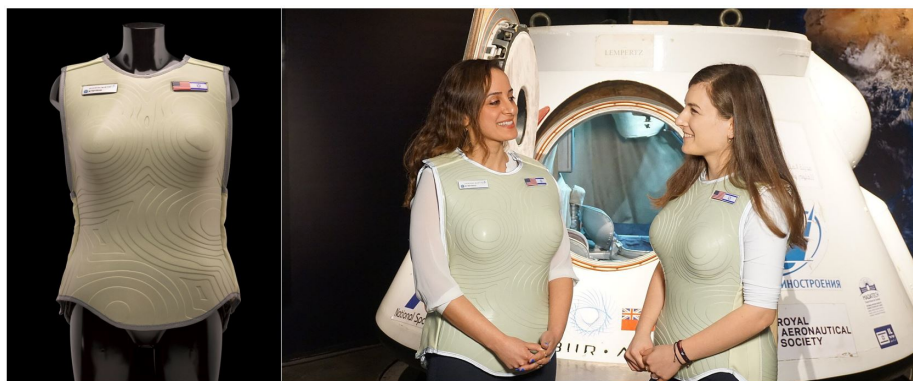
Figure 5: Left: The first prototype of the AstroRad vest, including a topographical design which shields better the tissues with higher sensitivity. Source: Lockheed Martin/Stemrad. Right: The second prototype of the Astrorad vest is expected to include materials inspired by pangolin scales. Source: Stemrad.
