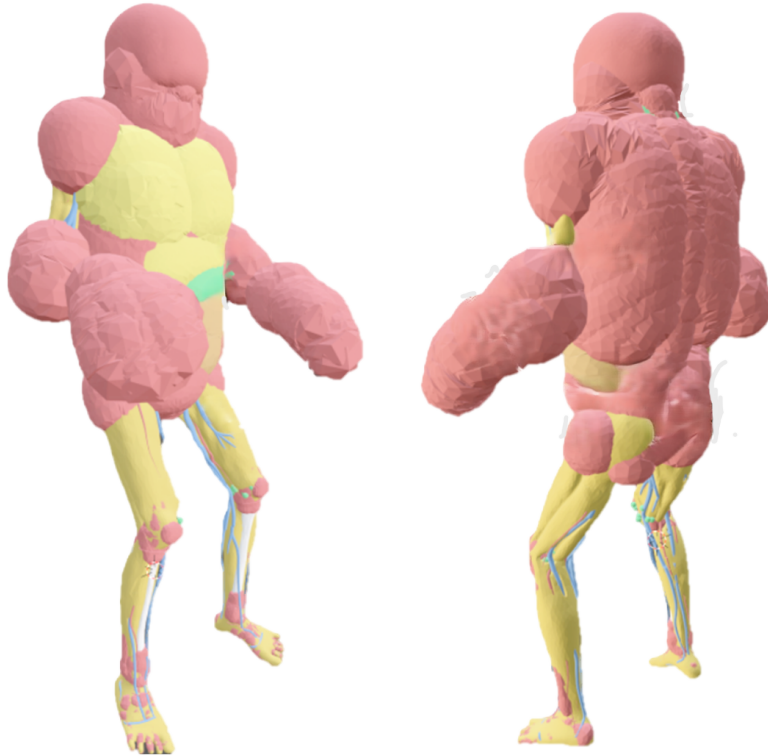
Figure 23: Visualization of the optimization case scenario where also tissues outside of the torso area would be allowed coverage by the suit. As the FLARE suit aims for torso coverage only, it is necessary to set suit thickness d = 0 for all such organs in the optimization algorithm, so that they do not add inaccurately to the effective dose reduction. †
