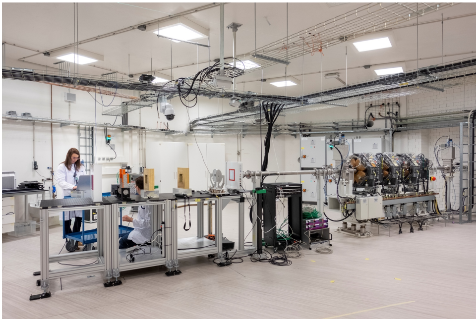
Figure 35: View of the R&D bunker at HollandPTC, featuring a fixed horizontal proton beamline from the ProBeam superconductive cyclotron for radiobiological applications. Source: HollandPTC.
