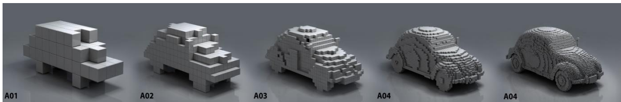
Figure 3.7: Different voxel resolutions, from low quality to high quality (Avin, n.d.)
