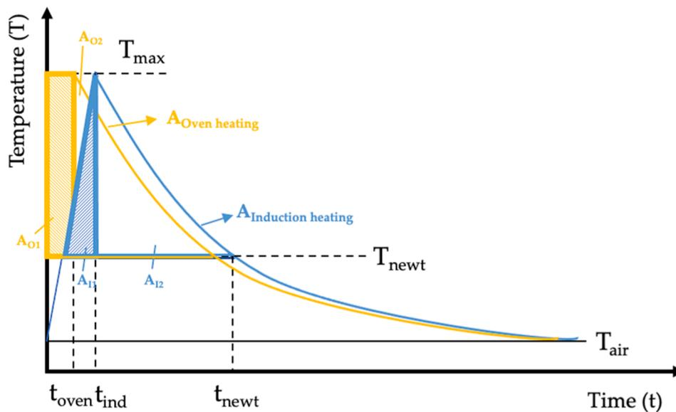
Fig. 5. Temperature changes in asphalt concrete by induction heating and oven heating.
