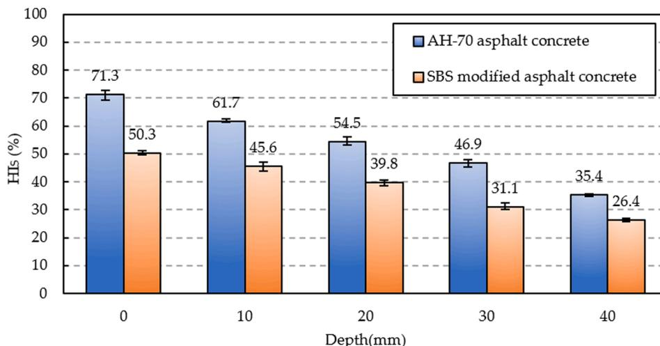
Fig. 9. HI<sub>s</sub> of AH-70 asphalt concrete and SBS modified asphalt concrete after oven heating.
