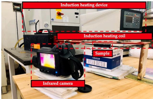
Fig. 3. System of induction heating test.
