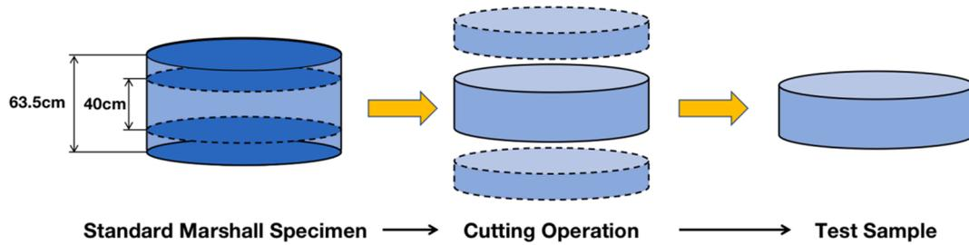
Fig. 2. Preparation of the samples in Induction heating test.
