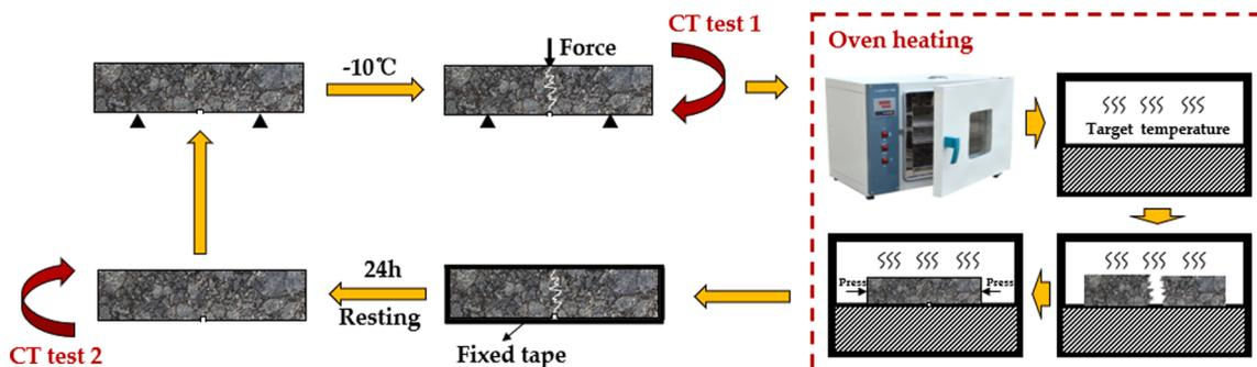
Fig. 4. Procedure of fracture-healing-fracture test.
