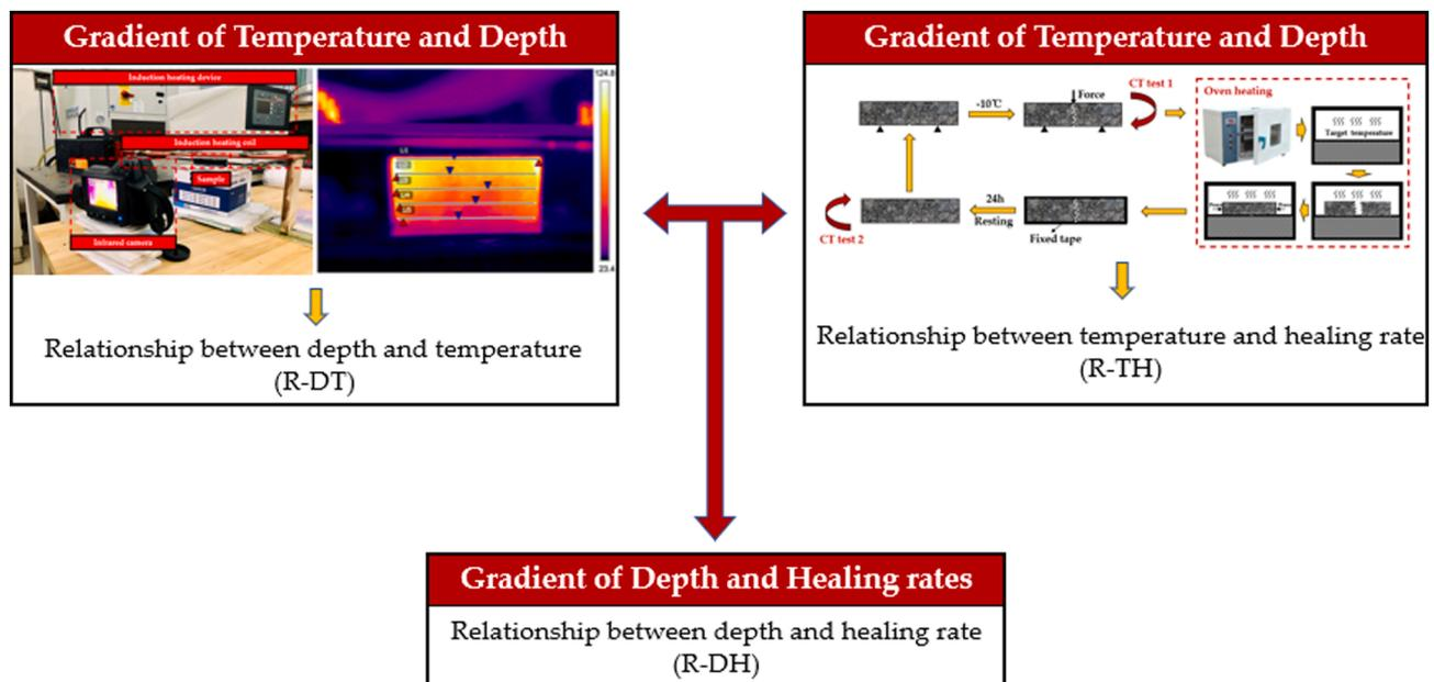
Fig. 14. Prediction method of gradient healing effect of asphalt concrete after induction heating.
