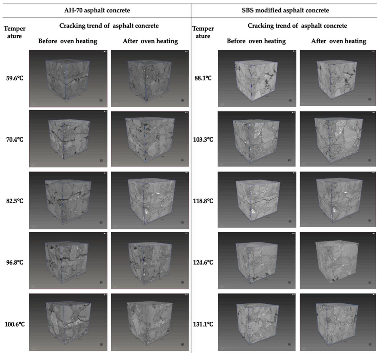
Fig. 11. Comparison of cracks before and after oven heating of AH-70 asphalt concrete and SBS modified asphalt concrete.
