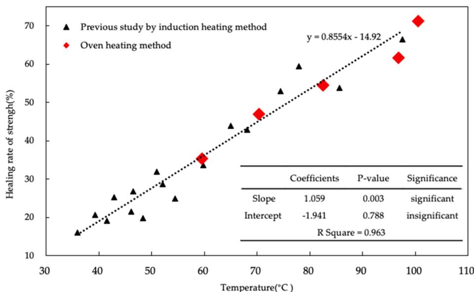
Fig. 10. Linear regression between oven heating method and previous study by induction heating method.
