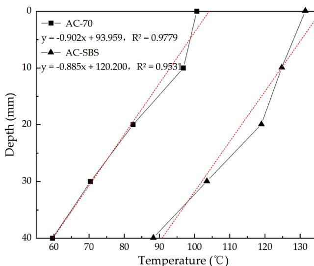
Fig. 8. Depth-temperature curve of asphalt concrete after induction heating.
