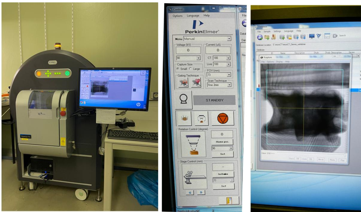
Figure 63 | microCT machine (left), microCT settings (middle), microCT preview (right)
