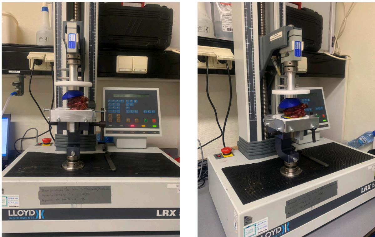
Figure 59 | CVB fracture creation process
