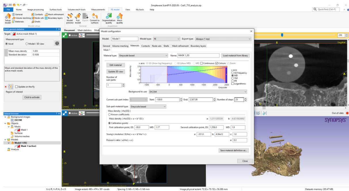
Figure 66 | scanIP HA Phantom properties setup
