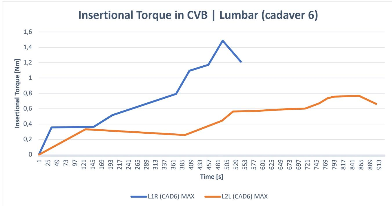
Figure 31 | Insertional Torque in CVB (lumbar, cadaver 6)
