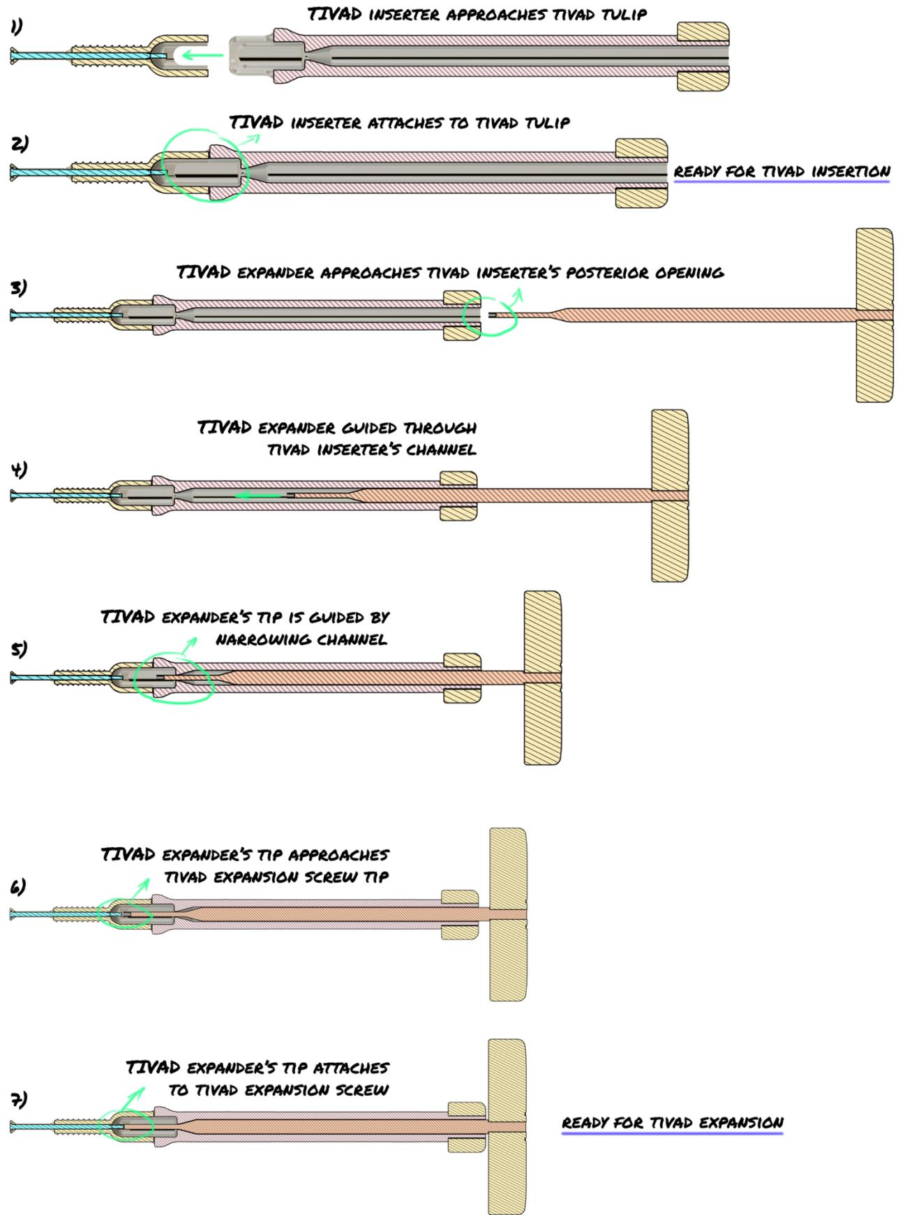
Figure 74 | TIVAD inserter & expander workflow
