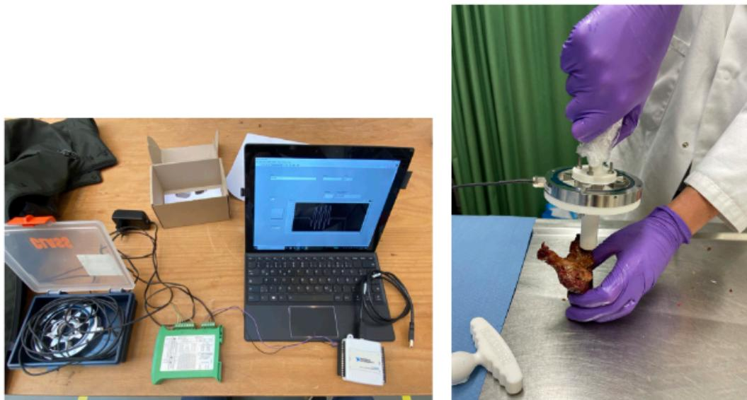
Figure 26 | Torque sensor setup: laptop, signal amplifier & DAQ unit (left). TIVAD adapter, torque sensor & Handle concept (right)
