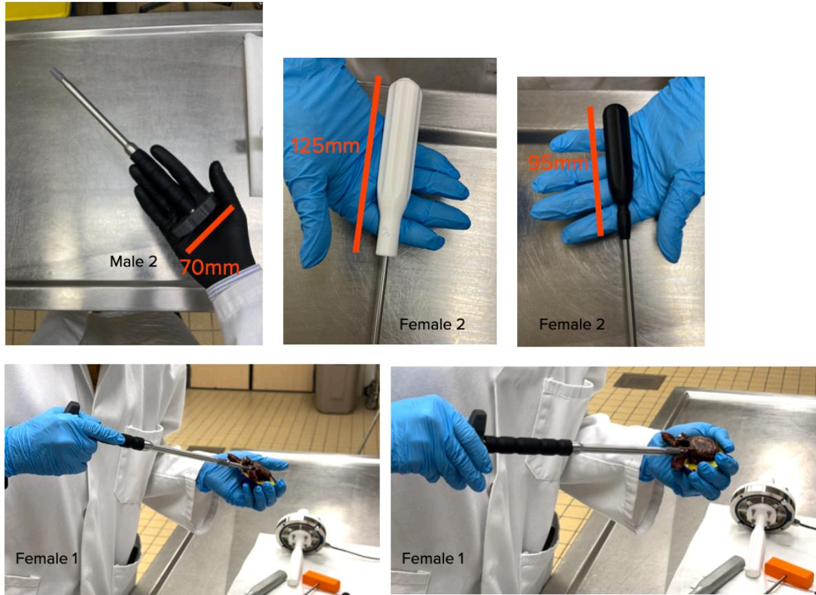
Figure 34 | Handle dimensions tests with different hand size
