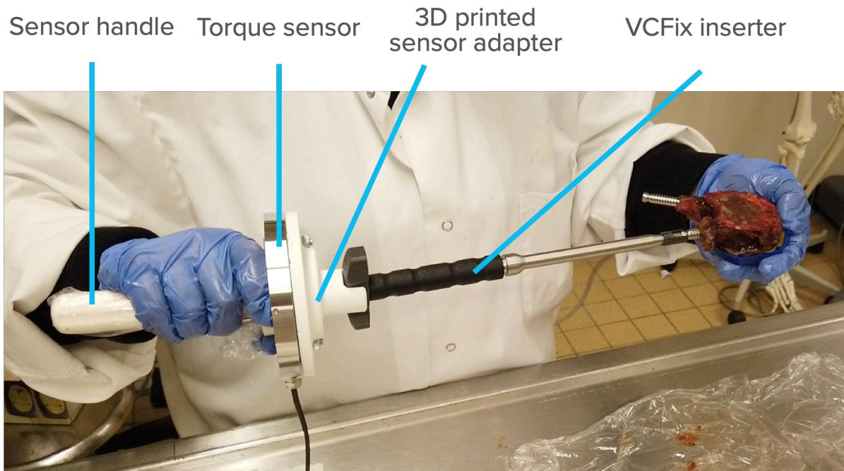
Figure 27 | TIVAD Inserter during stage 2A experimental test
