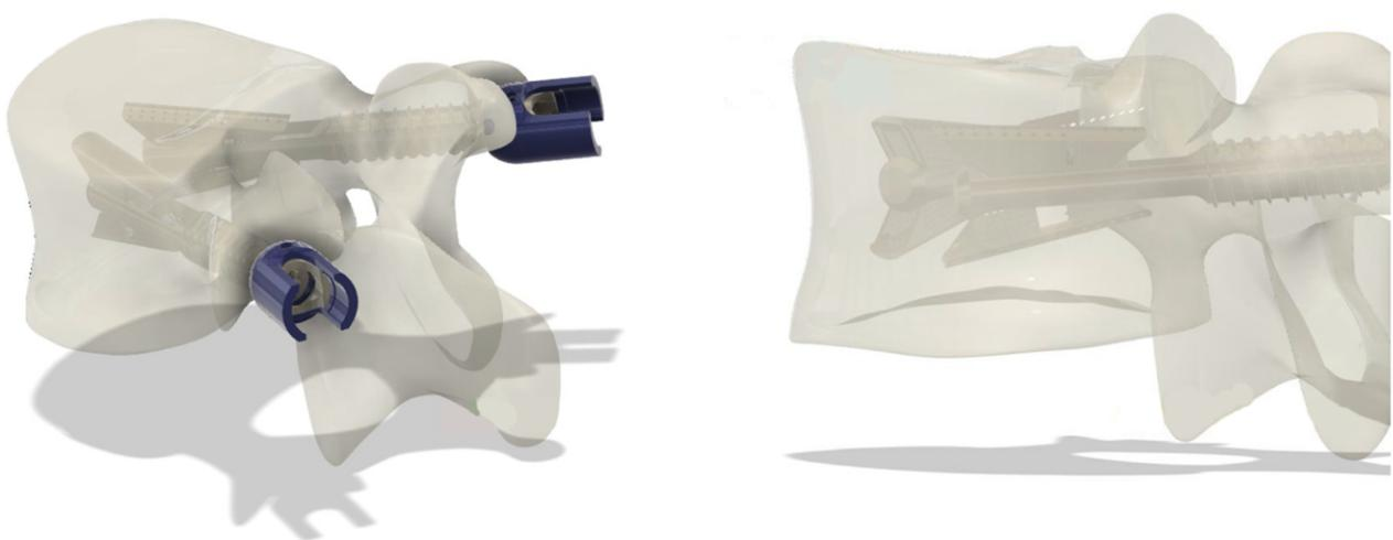
Figure 5 | In-situ situation of implanted and expanded TIVAD implant
