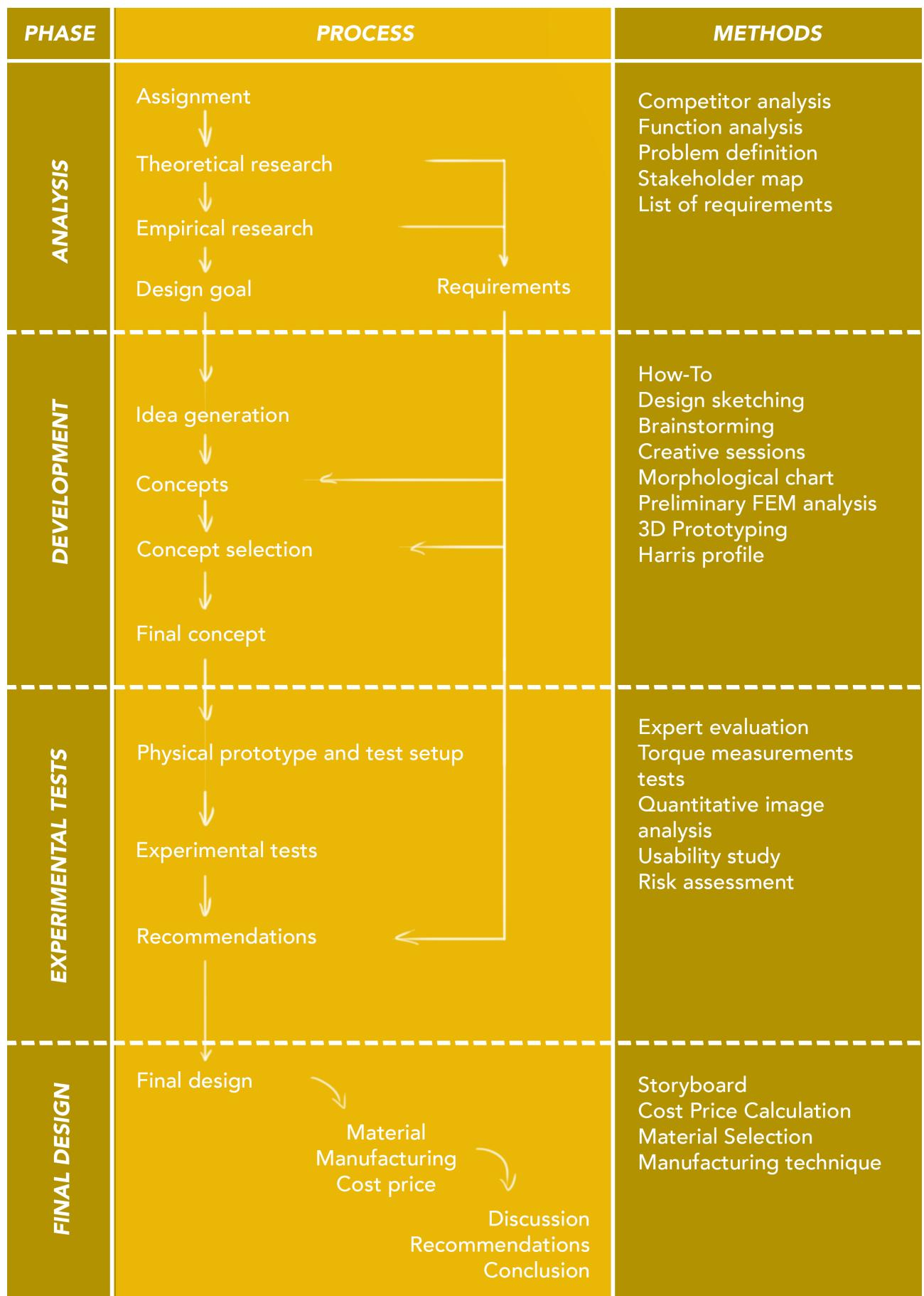
Figure 7 | Reader's guide of design phases, process, and applied design methods
