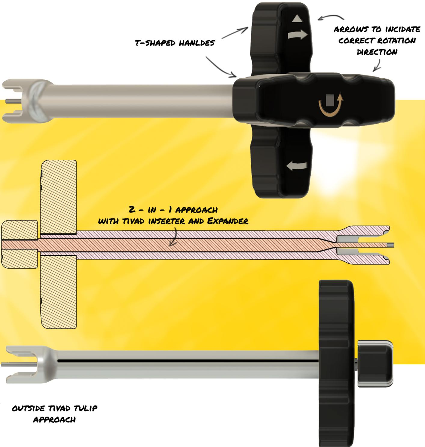
Figure 43 | Final TIVAD Inserter & Expander design
