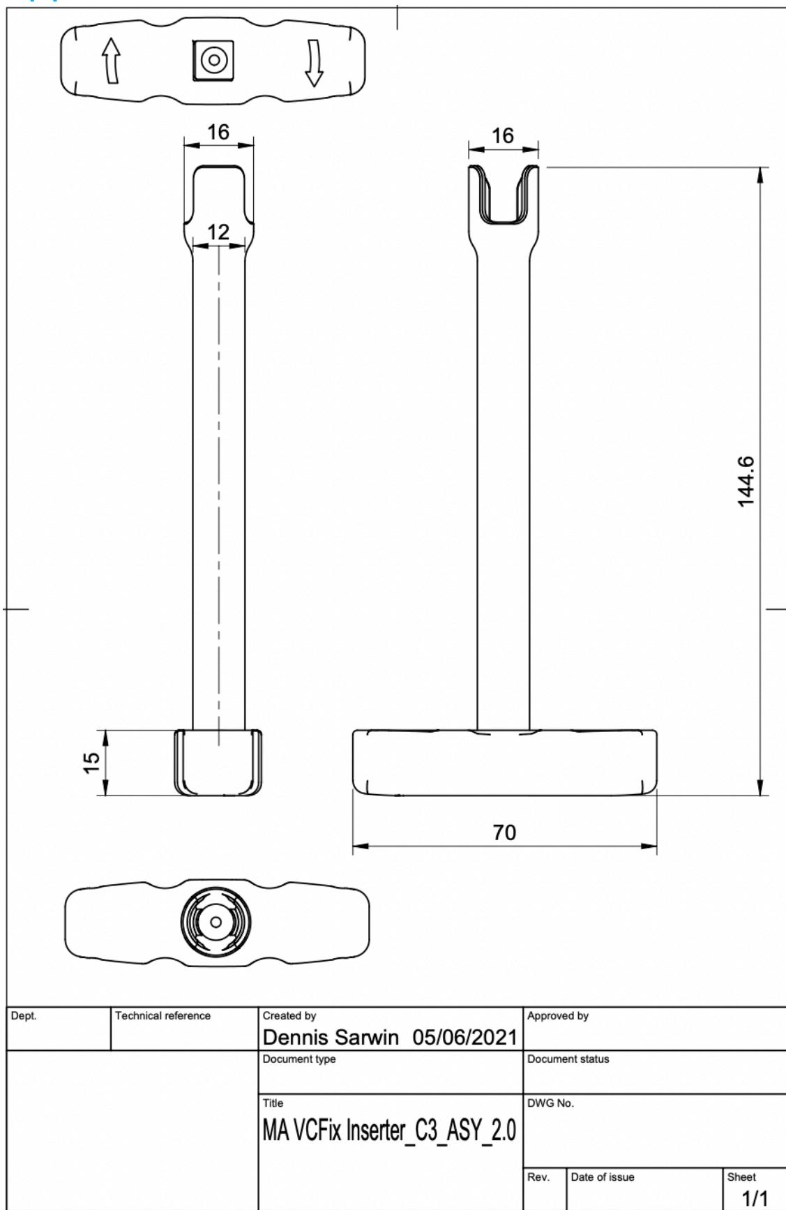
Figure 72 | TIVAD Inserter technical drawing
